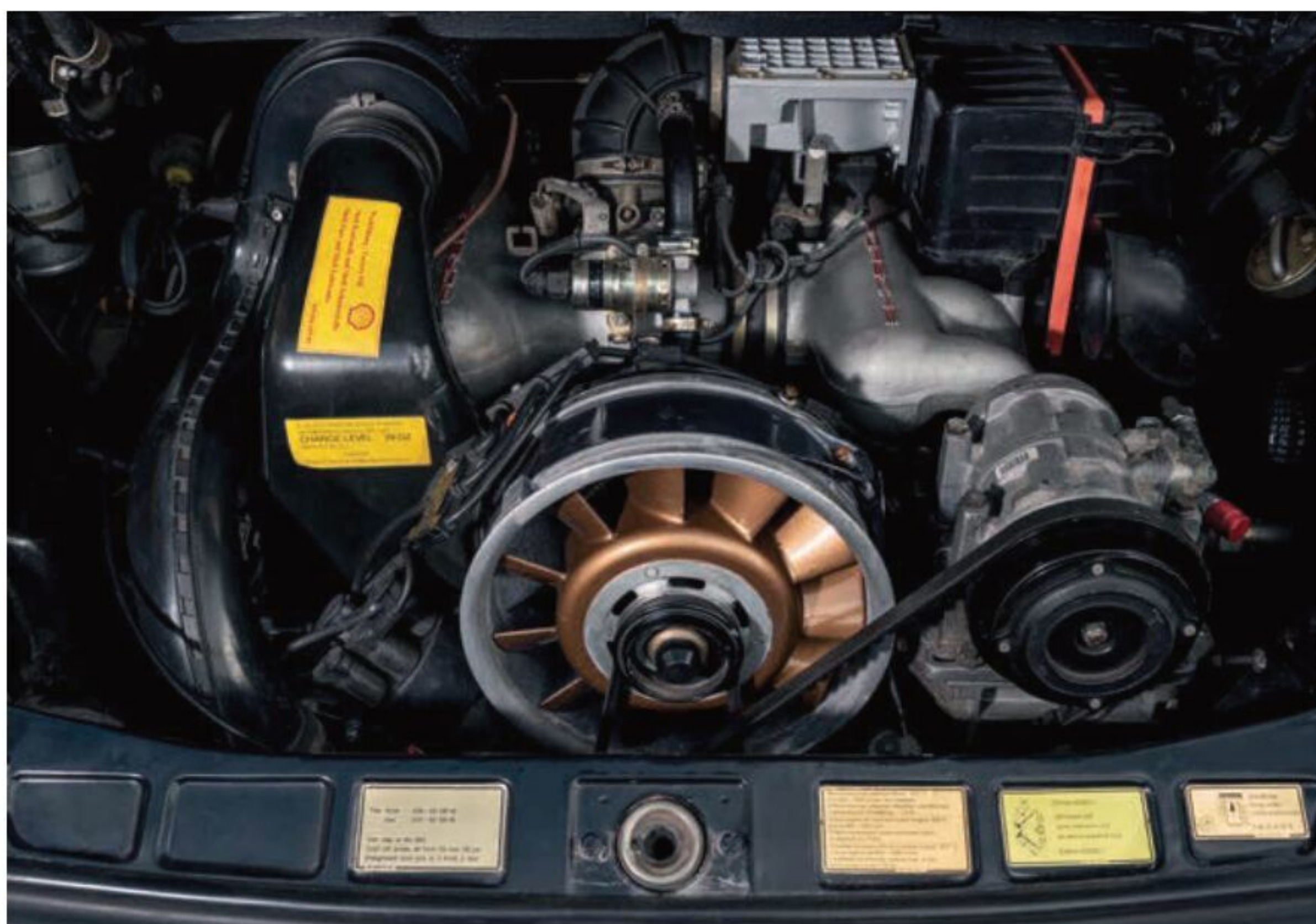
Above 3.2-litre flat-six is original to the car and has been thoroughly rebuilt
