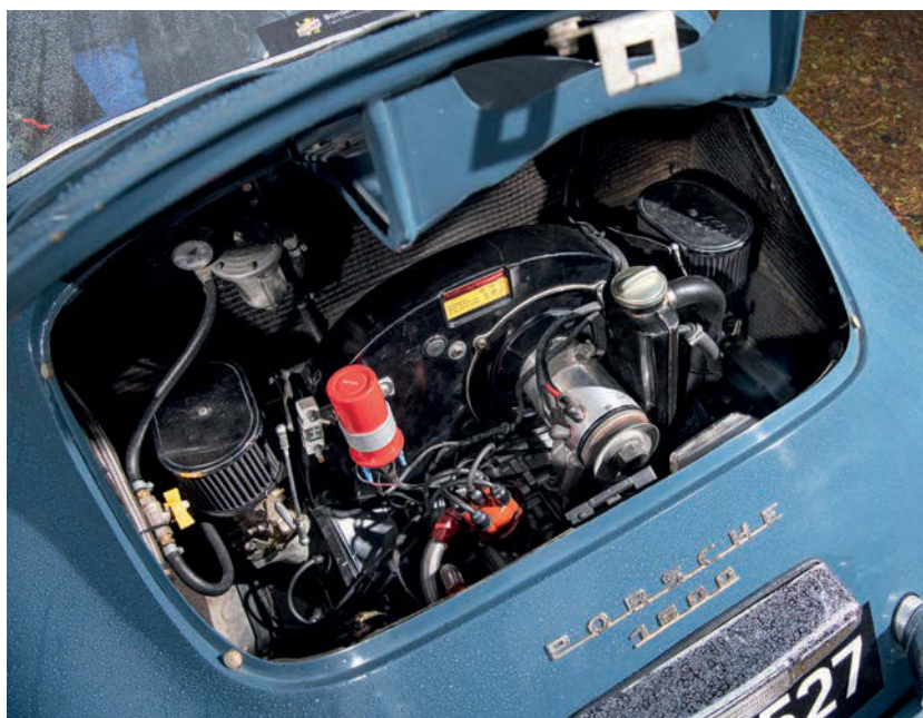
Above Rebuilt flat-four is producing 127bhp thanks to a tune-up from Anthony Seddon
