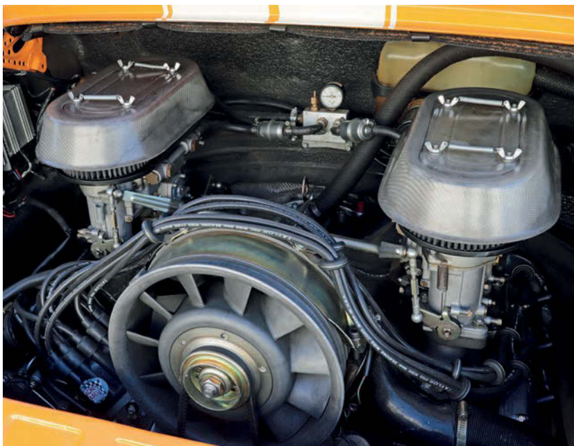
Above Flat-six has been enlarged to 3.4 litres, but makes use of carburetors instead of fuel injection
