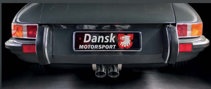
92.520DUAL / 1620610000 Exhaust, Sport, rear, 2 x Ø76 mm outlet pipe - TÜV/EEC approval
