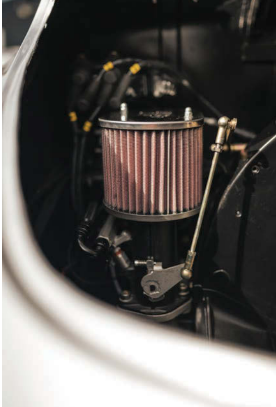
Above Jenvey DCOE-style Heritage throttle bodies and a DTA ECU work together to release 157 galloping ponies
