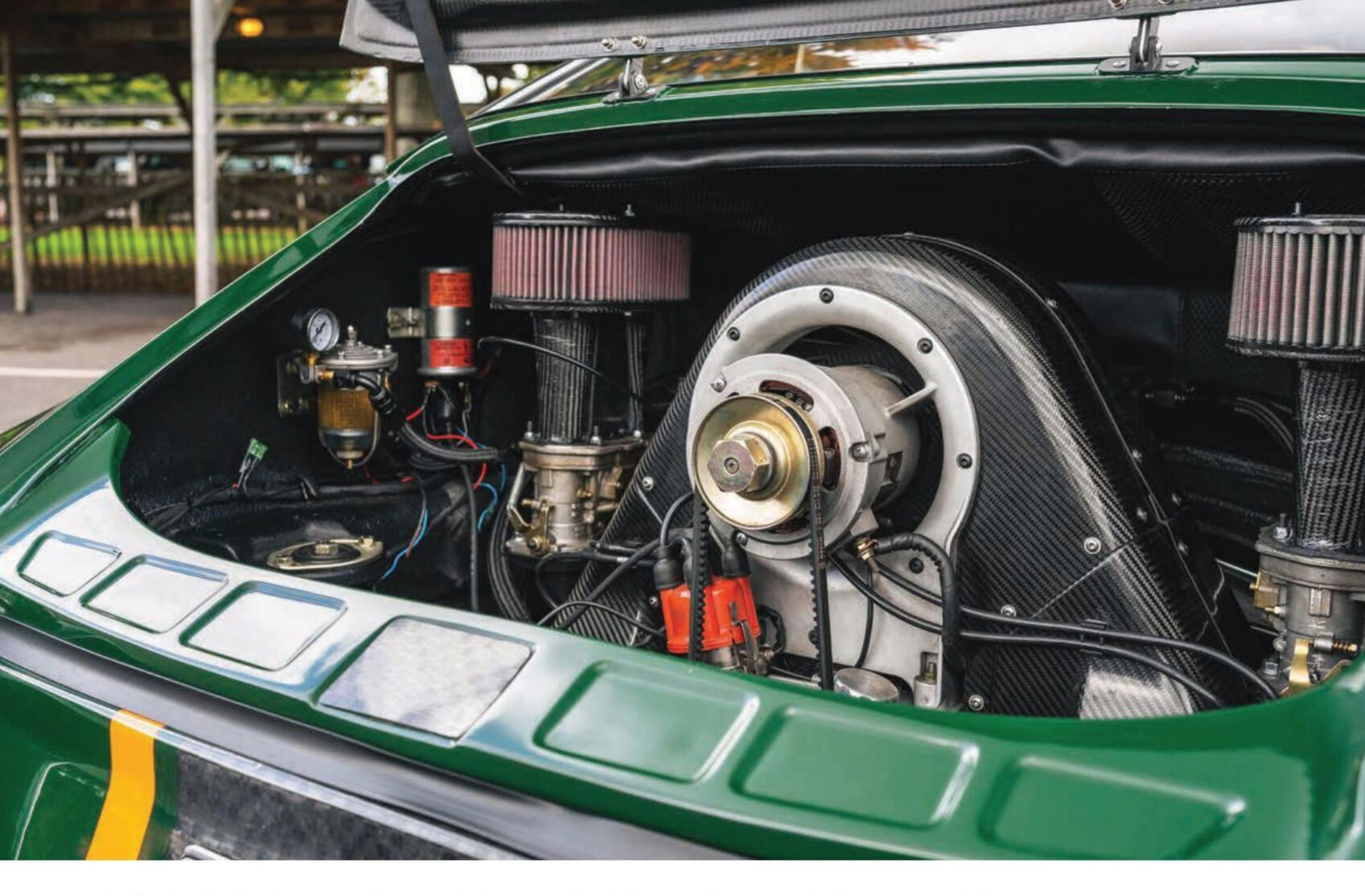
**Above** JPS Aircooled custom flat-four produces 170bhp and mimics the look of the Type 547 Fuhrmann four-cam
