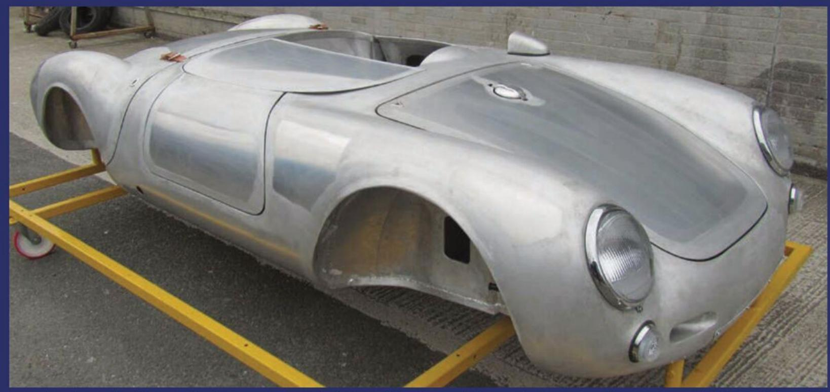
We manufacture Continuation Porsche 550's in the Original 3" Chassis Tube with hand made Aluminium bodies.
