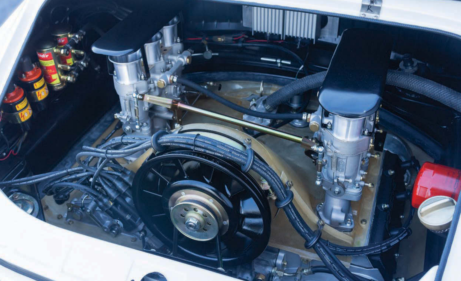
Above Gaspare's build is powered by a two-litre flat-six assembled along the lines of the unit found in the 906
