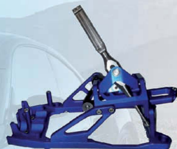
Multi Adjustable Short Throw Shifter for all 986, 996, 987 and 997
