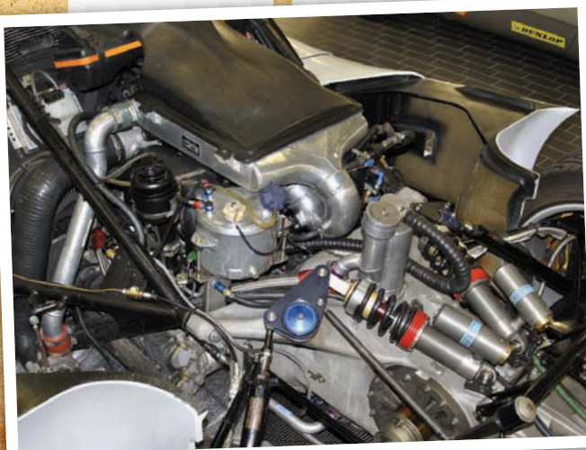
Ferry Porsche (below centre) was delighted when he examined the first of the street versions of the GT1. With the bodywork removed, pushrod rear suspension is clearly visible
