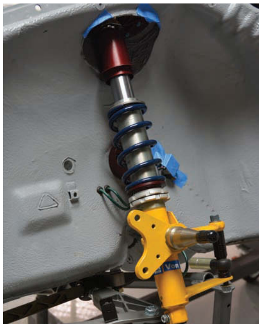
Below: Elephant Racing builds its own struts and dampers on site Right: Rolling bodyshell showcases the Elephant Racing product range
