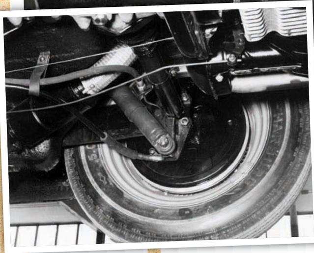
*The first major advance in Porsche braking came in October 1952 when Porsche fitted its 356 with these large cast-aluminium drum brakes, each fitted with a shrunk-in steel liner. Radial fins helped add strength and aided cooling*
