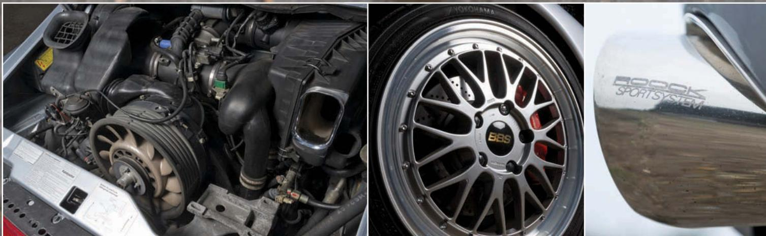
The 3.8-litre Cup engine is the real deal taken from a crashed Cup car. After some tweaking by Chip Wizards, it produces 318bhp and 310lb/ft of torque. BBS LM split-rims are a wheel design classic. Below: Lowered stance is spot on. Chassis set up by Center Gravity
