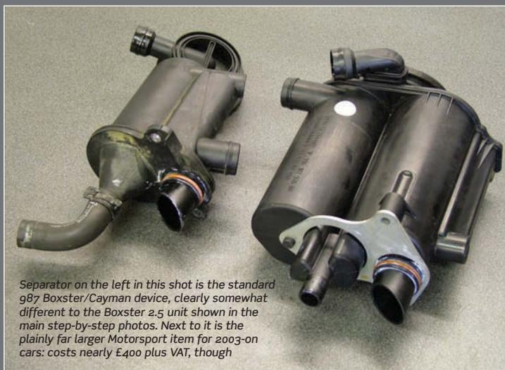
Separator on the left in this shot is the standard 987 Boxster/Cayman device, clearly somewhat different to the Boxster 2.5 unit shown in the main step-by-step photos. Next to it is the plainly far larger Motorsport item for 2003-on cars: costs nearly £400 plus VAT, though
