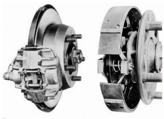
The annular disc brake is a fascinating design, with the caliper mounted 'inside' the disc. This allowed a larger-diameter disc to be used. However, the 356C (and the first 911) used this more conventional disc (right), which followed Dunlop's original layout, with an external caliper. A drum was located within the rear brake disc to serve as the emergency handbrake
