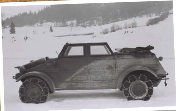
Above: Porsche designed a four-wheel-drive version of the Kübelwagen, called the Type 87. Right and below: Ill-fated Mercedes T80 Rekordwagen was a six-wheeler, with the four rear wheels powered by 3000bhp V-12 engine. 4WD allowed T80 to gain traction despite narrow tyres...
