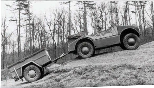
“By engaging a simple dog-clutch by pushing a lever, drive could be transferred to the front wheels...”
