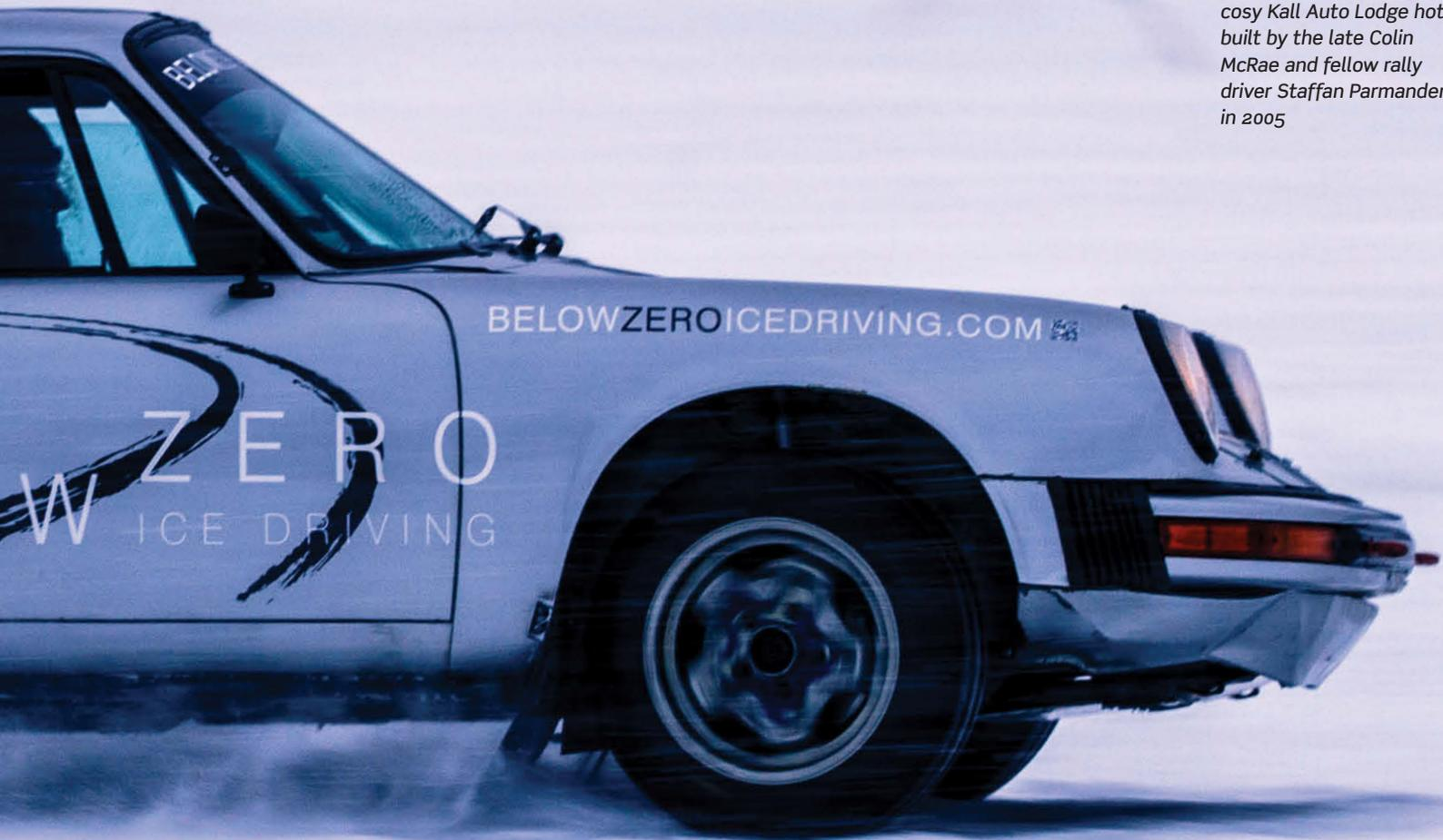
*The 911 of choice is the 3.0-litre SC for good reason. They're mechanically tough and can easily be tuned up to 260bhp. All have close-ratio gearboxes and limited slip diffs*
