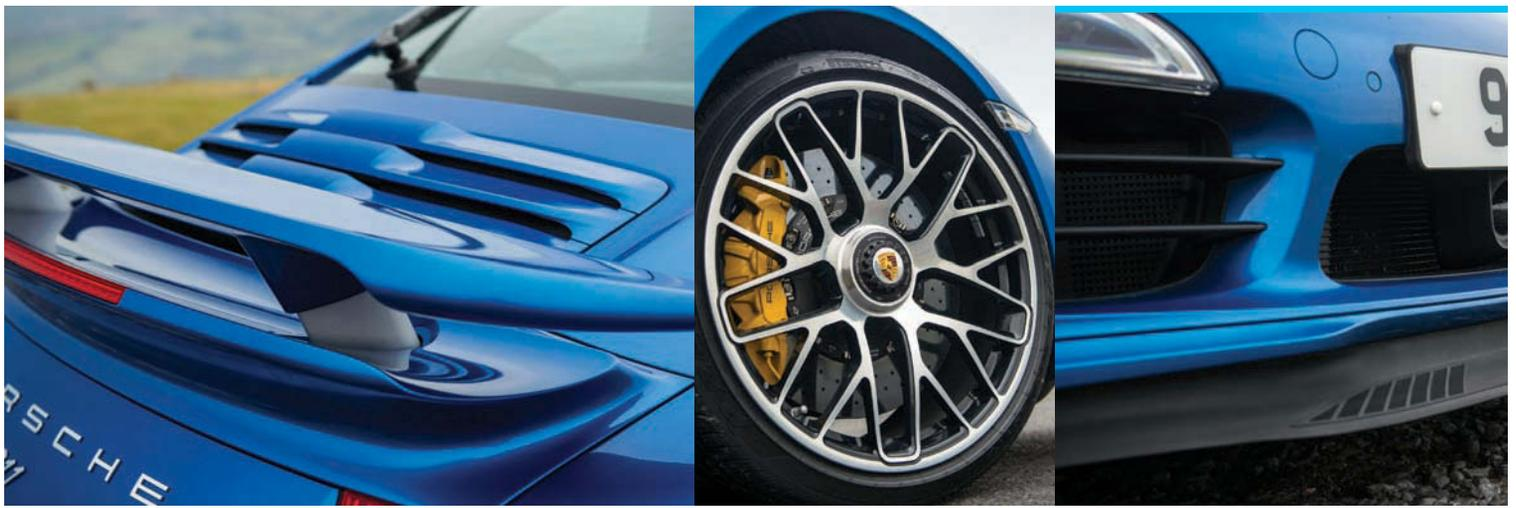
*Above and far right: Active aero in the form of retractable front and rear wings keep the new 911 Turbo pinned down at high speed. Massive 20in wheels accommodate 410mm ventilated carbon ceramic discs – standard issue on the Turbo S*
