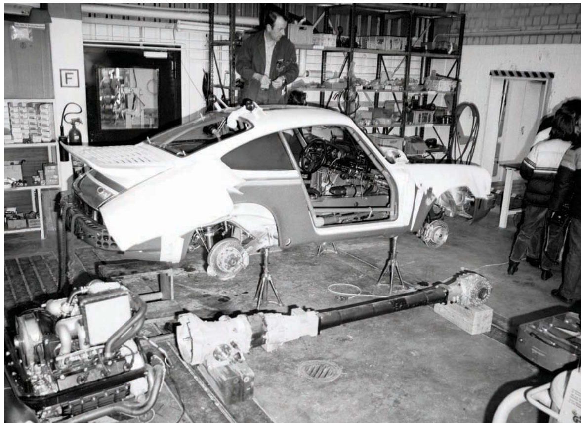
Below: The first of the Type 953 rally cars being prepared at Weissach. Note the torque tube connecting the modified five-speed Audi transaxle to the front differential
