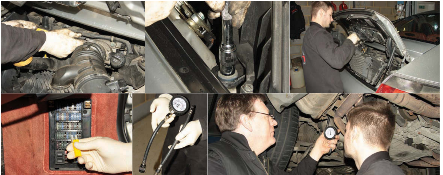
Inspecting all six bores requires slow and precise rotation of crankshaft to place each piston at the bottom of its stroke. Only safe way to do that is to remove the airbox for access to the pulley bolt. Compression check is carried out, with all six plugs removed, by spinning engine on starter motor - remove fuel-pump fuse to avoid petrol fumes. Flexible extension is essential to fit the Mg6's rather inaccessible plug holes. Consistency of readings as important as overall figure, here all about 11 bar
