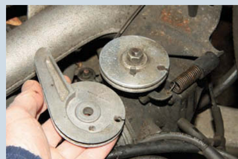
Eight-valve 944s had as standard this roughly snail-shaped throttle 'cam', but circular after-market device offers much better response
