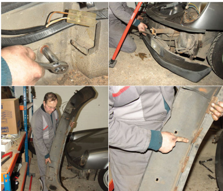
The start of our second dismantling session (or the third if you include the windows) saw the 3.2 minus its two doors, and about to be relieved of front and rear bumpers. Interior and headlining later followed, and then the front wings - both processes revealing major structural issues
