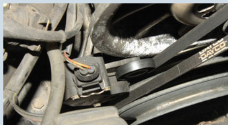
Plastic jockey wheel running against 993's (and 964's) cooling-fan belt (above, left) is designed to alert driver to the belt's possible breakage, but can itself fail and generate spurious signals. A popular modification, especially for power-tuned engines, is to lock alternator and fan shafts together (right) and use a single belt
