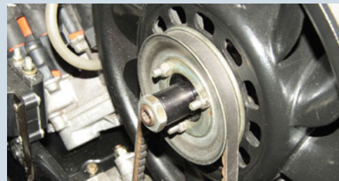
Plastic jockey wheel running against 993's (and 964's) cooling-fan belt (above, left) is designed to alert driver to the belt's possible breakage, but can itself fail and generate spurious signals. A popular modification, especially for power-tuned engines, is to lock alternator and fan shafts together (right) and use a single belt
