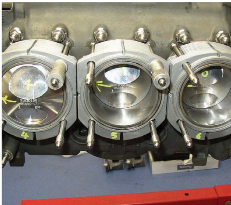
Above: 1mm-oversize forged Wossner pistons will give a compression ratio of 10.0:1. Above right: Stomski Racing supplied the mechanical cam chain tensioners used in preference to the stock design
