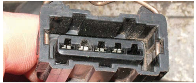
Our suggested diagnosis for Ian Milne's rough-running Carrera 3.2 proved to be spot-on: nothing more than a dirty electrical contact
