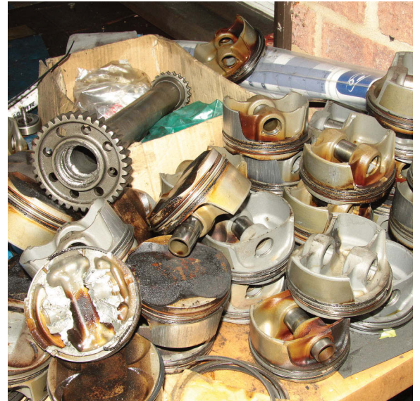
Northway's pile of scrap pistons – mostly from M97 3.6 motors – tells its own story. Most independents have something similar
