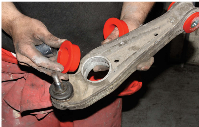
986 and 996 'coffin' arms are so called because, as you can see, that's what they resemble (above, left). It's the ball-joint at outer end that causes that annoying creaking; this one is also being fitted with after-market Polybushes (see the July 2011 edition). Changing rear arm (right) will entail a 'geo' check: pivot bolt (arrowed) adjusts camber
