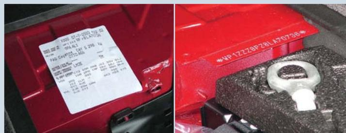
2008 Cayenne's VIN - stamped into cargo-space floorpan - shows type number, like that of first-generation cars, to be 9PA; VIL (left) shows additional AL1 code
