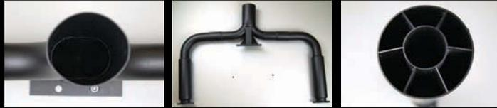
Manufactured in the US, European Racing Headers are made from equal length, mandrel bent 16-gauge mild steel and are a three-into-one configuration. They bolt on with no modifications necessary.
