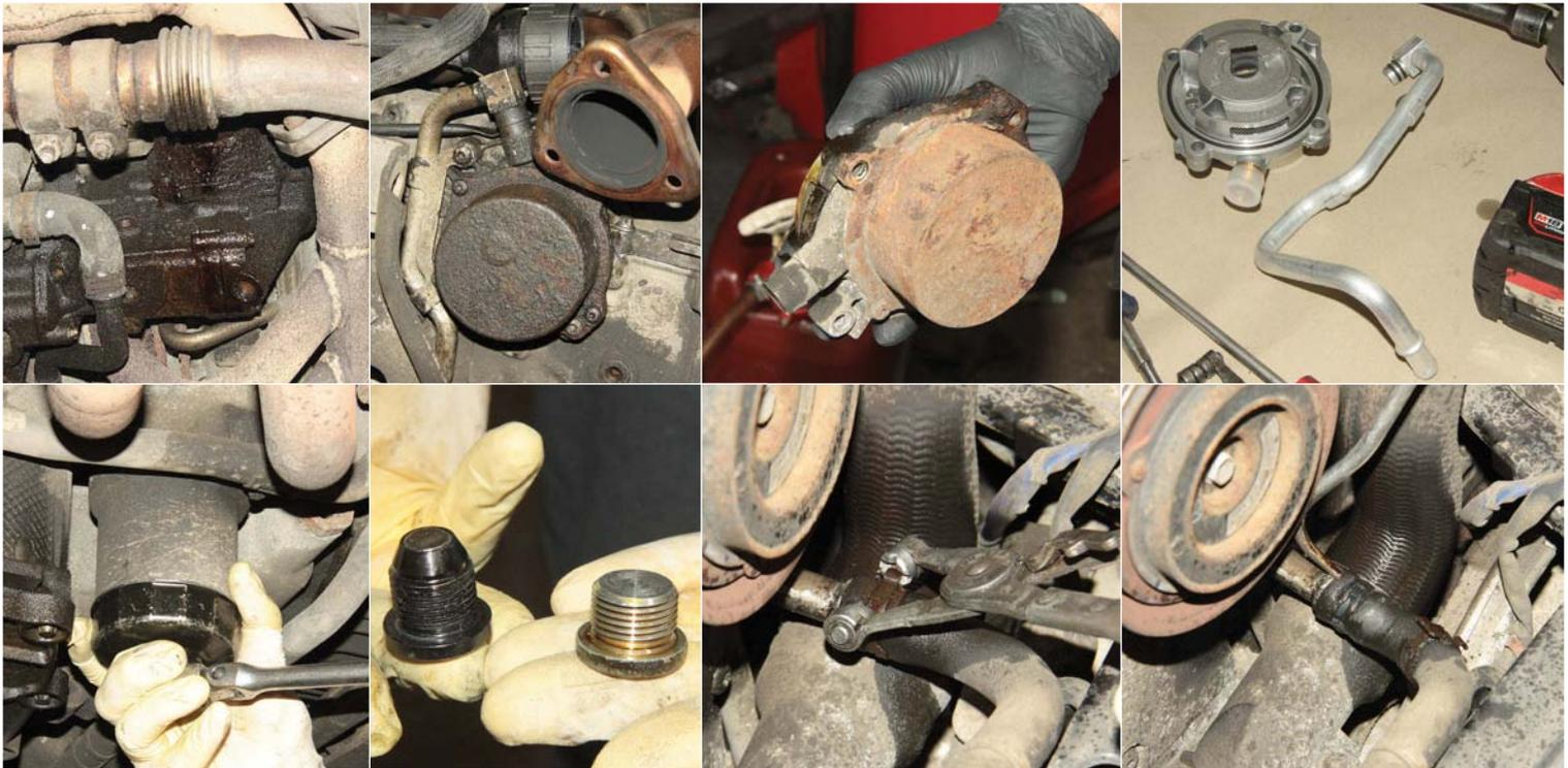
Access to pump necessarily limited; second pic from top left shows its location on another engine, removed from car. Surface rust quickly develops into tiny holes. New pump costs £318 plus VAT. Job requires draining engine oil, so a good opportunity to change it, together with filter; install magnetic sump plugs, too. Remove air-filter housing for access to top end of metal pipe
