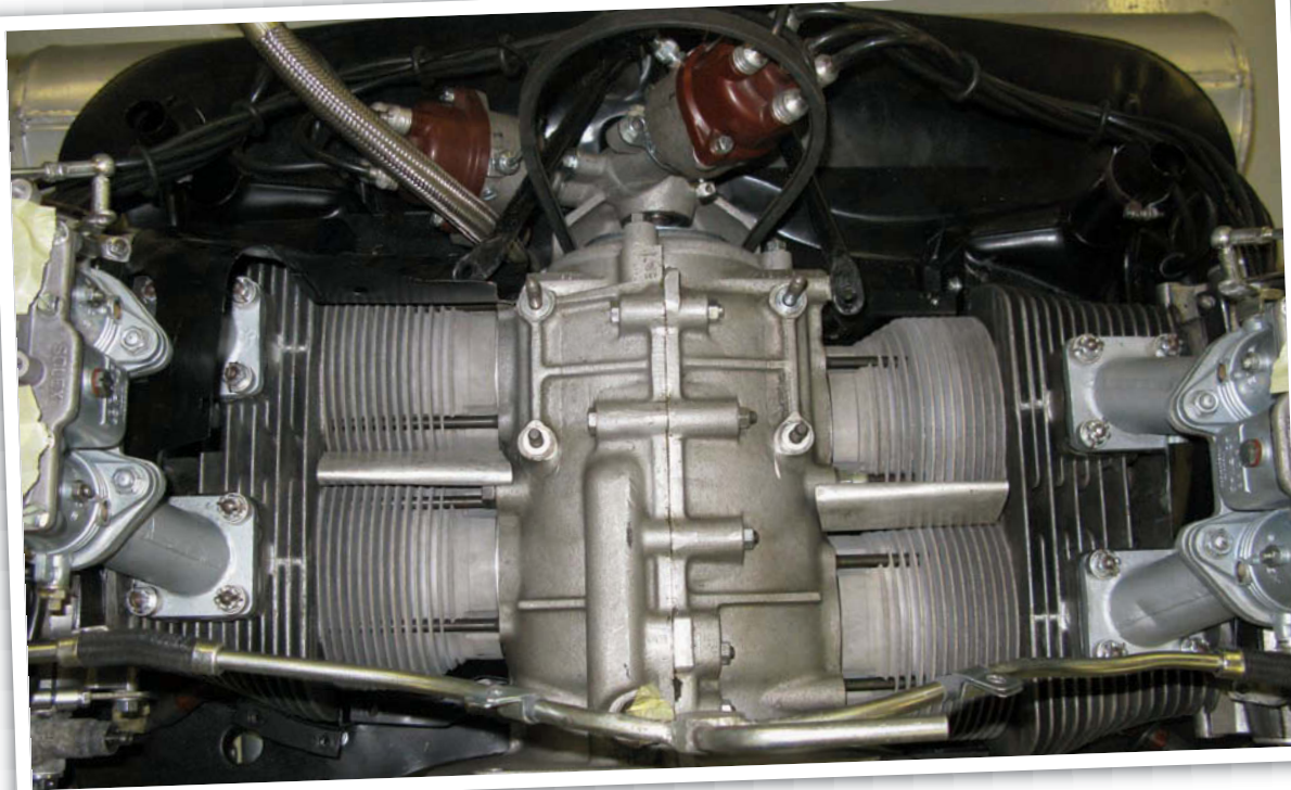
Left: Viewed from above, with the cooling shroud and fan assembly removed, it's possible to see how substantial the four-cam's engine case is. Cylinders are cast in aluminium with plated bores
