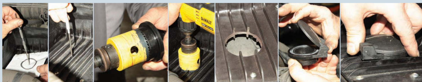
Paper template helps find the spot; that is then 'found' again with a scribe, and a very small pilot hole can be drilled. Hole saw needs to be exactly the right diameter; extract plastic swarf with a vacuum cleaner. Making sure valve is correctly seated, position it so that the flap can open beneath the air filter; otherwise it's useless
