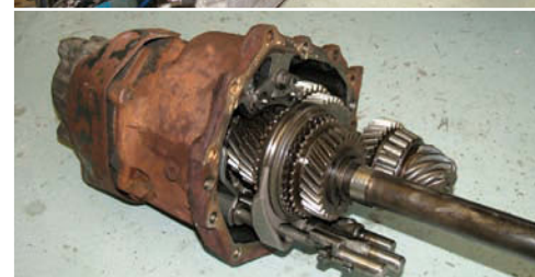
Output-shaft bearings in Horton's 944 were badly worn and commensurately noisy, but replacement was relatively straightforward – if you call removing and stripping the transaxle straightforward, that is
