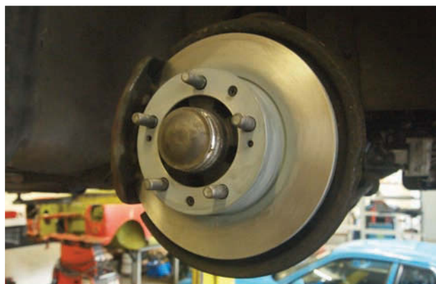
Below: New front discs and pads have improved the braking. Rears next. Rear Konis in situ attached to the swing arms. No springs? No, the 944 uses torsion bars at the rear like the pre '89 911s. Gearbox and everything else removed for clutch swap
