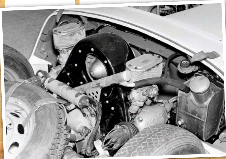
Below: Seen here in an early Type 550 Spyder, the Fuhrmann-designed engine relied on dry-sump oiling - the oil reservoir can be seen to the right of the engine. Note the rear-facing distributors in this mid-engined installation. Large cooling fan pulled in air from both sides of the shrouding
