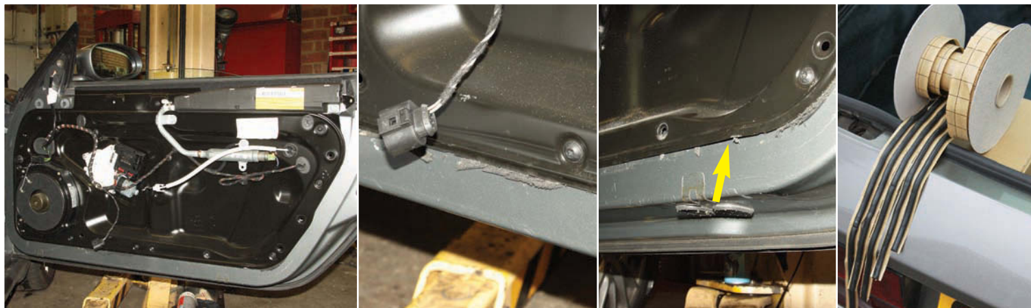
Like many current and recent VAG vehicles, 987 Boxster/Cayman and 997 Carrera have a pressed-steel 'component carrier' inside each door, behind fabric trim panel. It should be sealed against the door shell by a foam-rubber strip, but that eventually perishes (middle two pics) and allows water into the cabin. Strictly correct fix is a complete (and expensive) new carrier, but buy some mastic-style 944 rear-light sealing 'cord' (far right) and you can at least have a go at reclaiming the original panel
