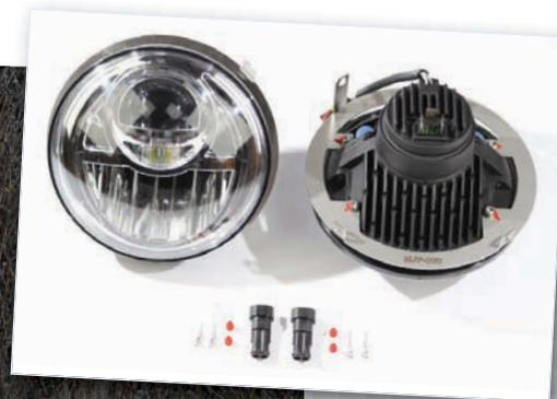
LumeTechnik (above) is an easy installation in all air-cooled 911s up to and including the 964. Special laser-cut brackets allow the units to fit quickly and neatly inside the standard headlamp covers. Only the sidelight wiring requires minor modification. It's never easy to show in a photo how good any light might be, but RPM car (left) amply demonstrates the whiter and crisper light the system delivers. Another big plus is the minimal heat generated by all LED lamps
