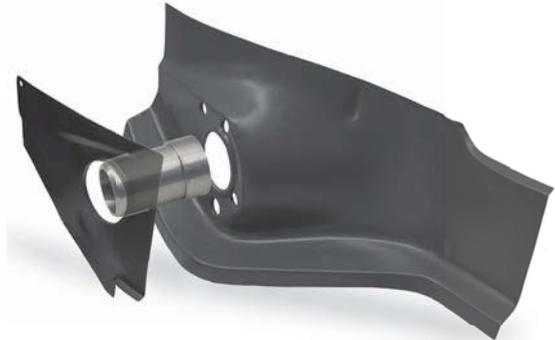
**Heating tube inside sill left and right**
