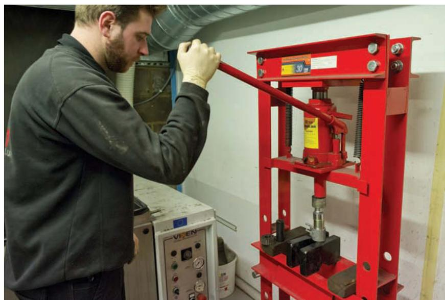
Left and right: A bench press is essential for the task of removing and pressing in new bushes
