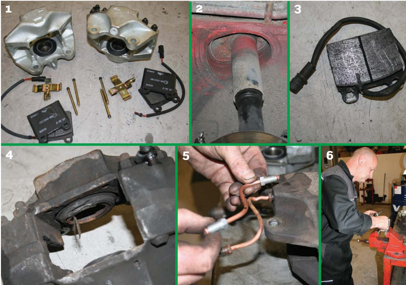
1) New kit. Shiny ATE remanufactured calipers come with new pad retaining clips and pins. Pads from Design 911 are manufacturer's original equipment, also from ATE
