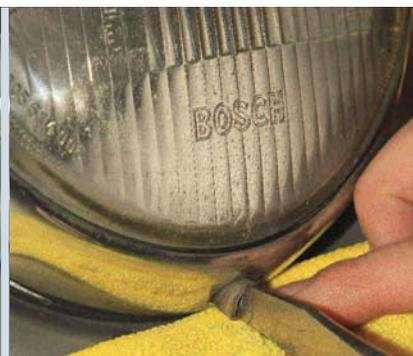
Standard headlamp glass has a chrome-plated trim, and perhaps a body-coloured trim over that (far left and middle). If the latter, undo the fixing screw at the 'six o'clock' position, and then in both cases the further larger screw securing the entire lamp assembly to the recess within the front wing. Cloth protects paintwork
