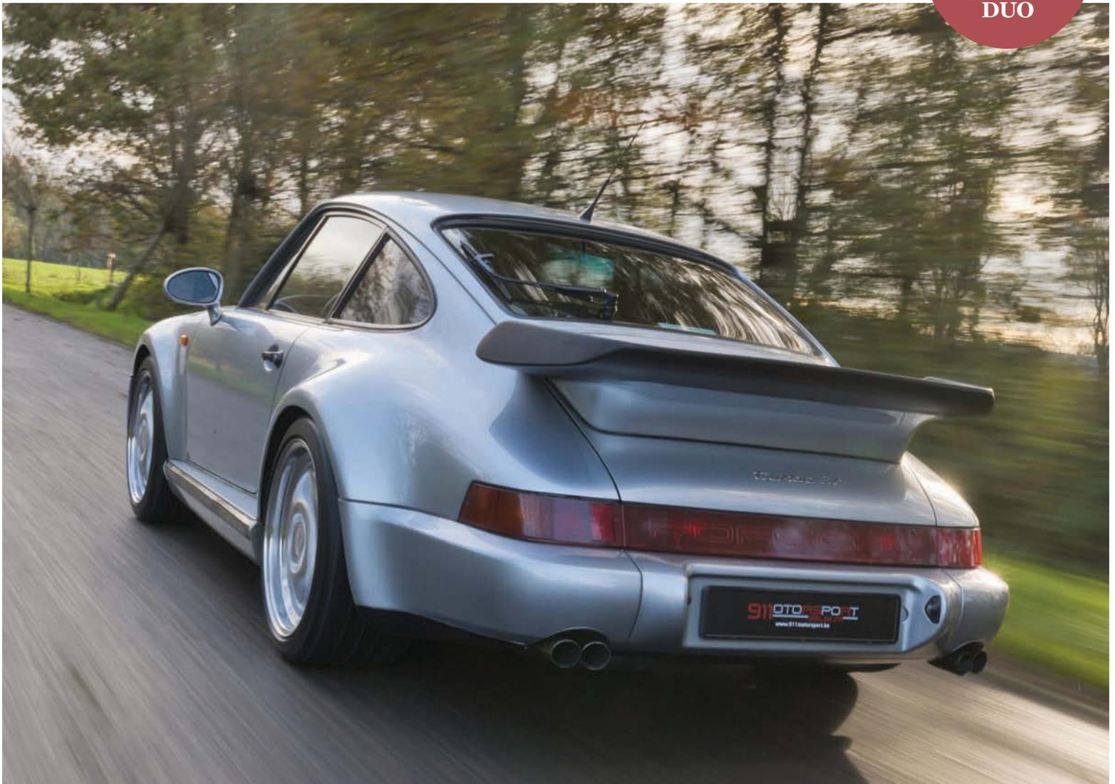
protruding beneath it. Mirrors are teardrops, and much of the core of the bodyshell is regular 964, but the extremities are different. The Turbo tea-tray rear wing contains the intercooler.
