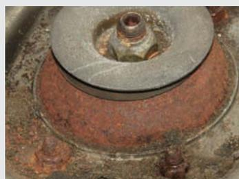
The four nuts and studs securing 924/944 suspension struts to the front wings often corrode quite badly, with the problem seemingly worse for the inboard pair each side, due to rainwater and condensation pooling around them. The solution – if absolutely necessary – is to fit replacement bearing flange(s), as they are known, but since those are no longer available from Porsche that will probably entail buying complete second-hand struts; see text
