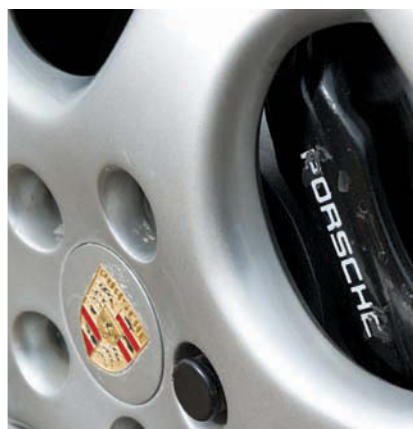
Left: Distinctive and huge intercooler sits on top of the 964's 3.3-litre, air-cooled flat-six. Power is 320bhp. Clocks are resolutely analogue, while four-pot alloy calipers were considered huge for 1990
