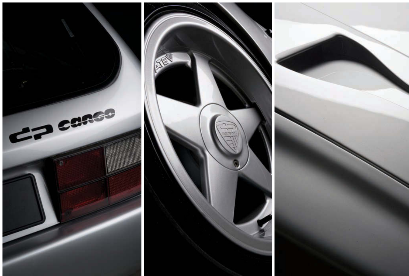
Left: DP Motorsport logo is familiar, while 'cargo' logo is typical of the period. Deep dish AZEV wheels have always suited the 924/944 well. NACA duct in the bonnet feeds intercooler
