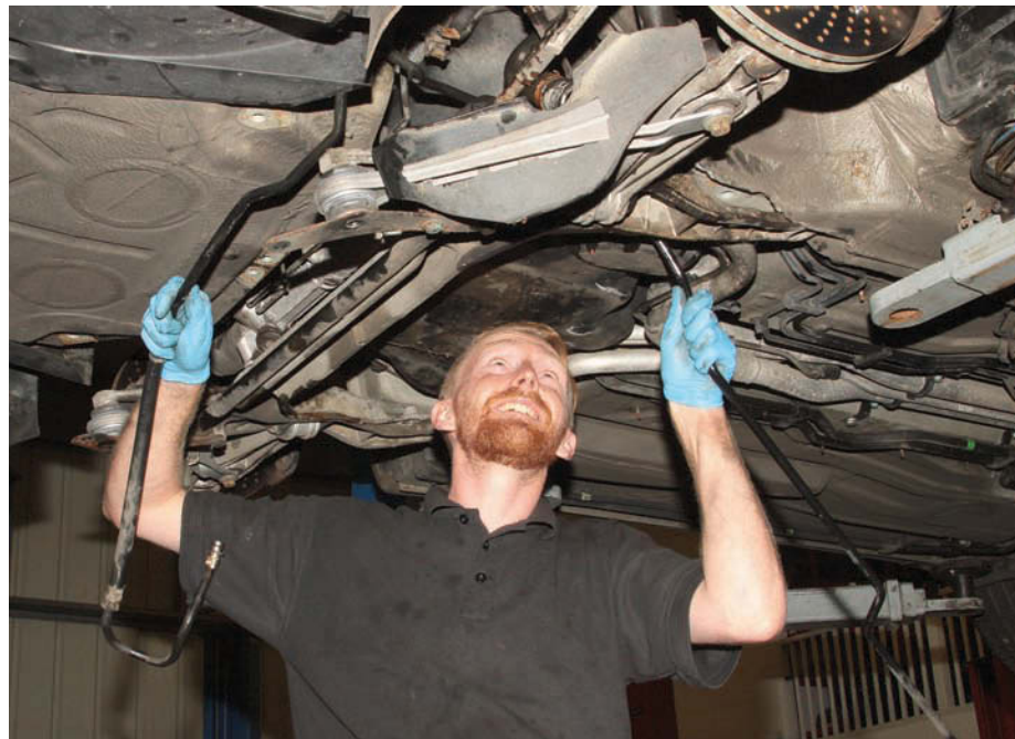
We showed how to fit 996 steering-rack pipes in a recent technical story (above), but reader John Barker has so far been unable to buy the correct lines for his Carrera 4. As yet we have no satisfactory answer, but we're on the case. In the meantime our suggestion would be to have them made by a specialist hose fabricator, perhaps with flexible sections that would make them far easier to install than the OE items
