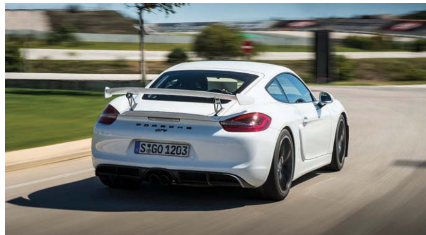
Cayman GT4 sits fully 30mm lower than standard car. Wheels are straight off the 911 GT3, as is entire front suspension and massive brakes
