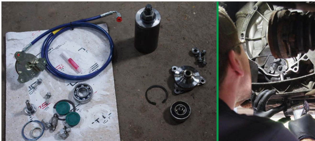
Left: The complete TuneRS Motorsports Direct Oil Feed kit. Note the open bearing for constant lubrication. Old sealed bearing to the right. Fitting is a big job, involving removal of the gearbox
