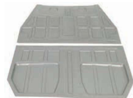
Floor Pan Parts For all 356, 911 and 912. We have all required panels from the front trunk and battery box back to the rear floor—including all required mounts.
