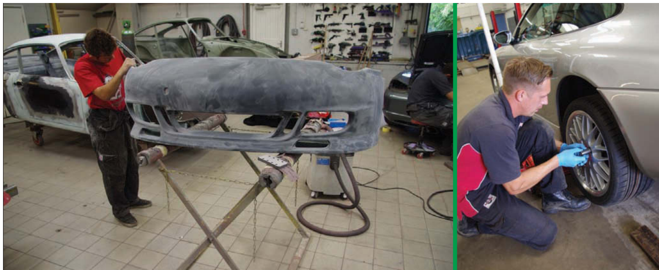
Left: New front apron receives prep and paint at Norfolk Premier Coachworks. New wheels and ContiSportContact tyres being fitted at Kingsway Tyres
