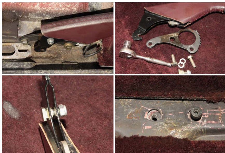
944's handbrake is a simple mechanism, easily removed and dismantled for lubrication. If you take out the seat, make sure that all fixing holes are undamaged – and use only the right screws to refit it
