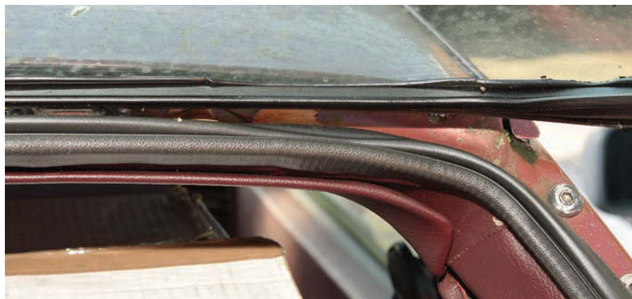
Horton changed his 944's tailgate seal, primarily because the old one had become completely flattened at its top corners – but this was the new one after only a few days. Was it worth the effort and expense?
