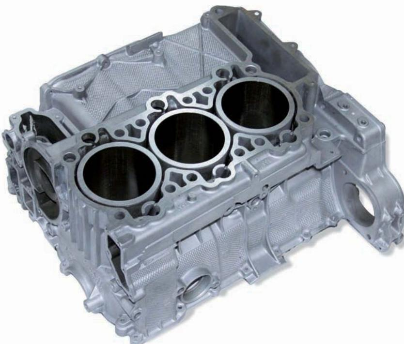
Block pictured left is from LN Engineering in the US; one of its well-known 'Nickies' conversions, which are also available – in a rather different form, of course – for air-cooled 911 engines. Note retention of open-deck block-to-head face, for what the company says is optimum cooling
