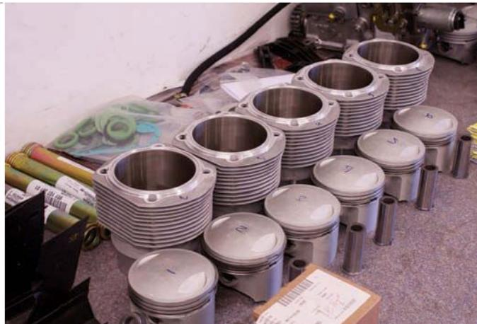
conversion projects. 'We aim for 100bhp per litre, and without creating a peaky engine,' he beams. 'With our 3.5-litre conversion for the 3.2 we twin-spark the engine, almost like creating a little RSR, which helps give us 350bhp.'
