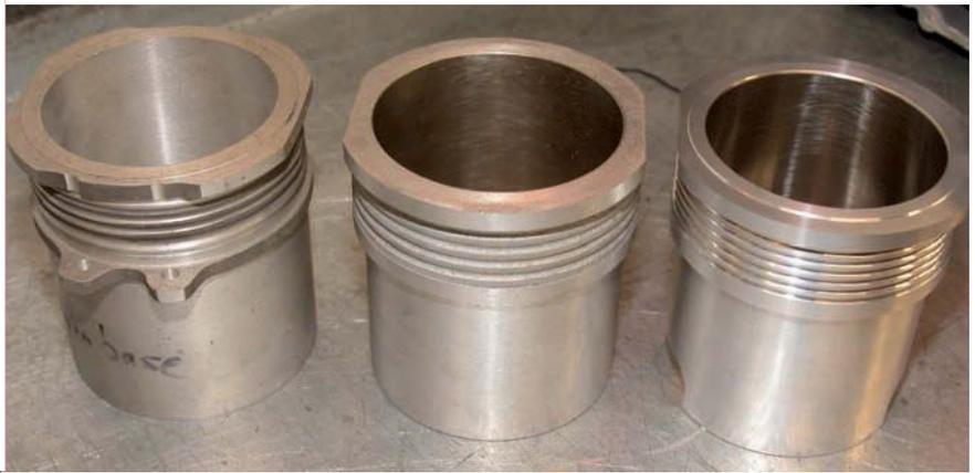
answer was Lokasil, which as its name might suggest is basically a rather more localised application of a silicon-based cylinder-manufacturing technique within a cylinder block that can as a result be made from a softer and less specialised material.
