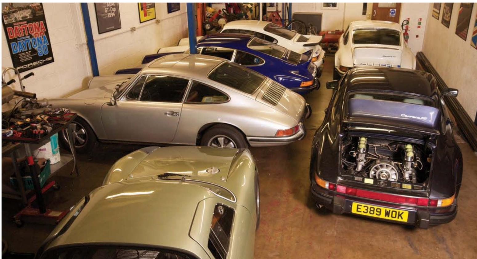
Engine conversions are a hugely popular part of Redtek's business. 3.2-litre engines are taken out to 3.5-litres, with twin-plug heads to give 350bhp. 964 engines can be taken out to 3.8-litres, with throttle bodies, cams and bigger valves, to give 350bhp
