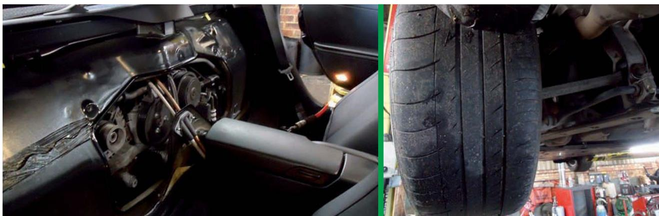
Left: So that's where the engine is! Interior panel removed to change drive belt. Rear Michelins have covered 17,000-miles, with another 5000 miles of life left in them
