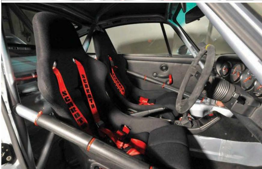
Top: Split-rim BBS wheels are the ultimate extra for an RS of the 993's era. The Club Sport is pretty much a road registered racer, as borne out by the stripped out interior and welded in cage
