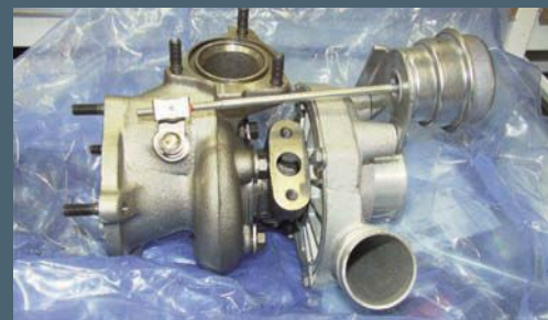
Corroded actuating rods culminated in a pair of brand-new turbos (among much else), and a VERY big bill...
