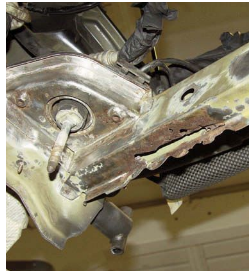
Precisely why this 997's rear crossmember has rusted in such a spectacular fashion is open to question, but roasting from nearby 'cats' is the most likely cause
