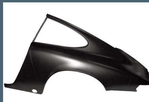
The huge range of top-quality repair panels from Dansk has been joined by this complex fuel-filler surround (left), and what might be termed a partial rear wing, designed to be cut into smaller sections, as necessary
