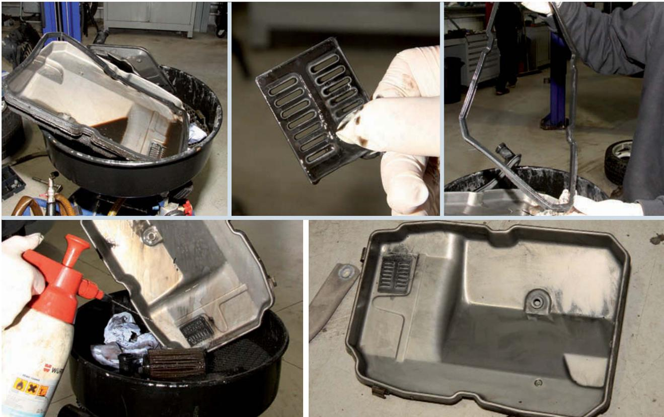
It should be a very simple matter to degrease and clean the sump pan, both inside and out, but note this internal magnet (top row, middle photo), designed to trap ferrous particles within the fluid – so don't be too alarmed if you see any; that's entirely normal. (How many are too many? You'll probably have to use your own judgement for that, but seek professional advice if both the magnet and/or the fluid seem especially contaminated.) Discard the old gasket
