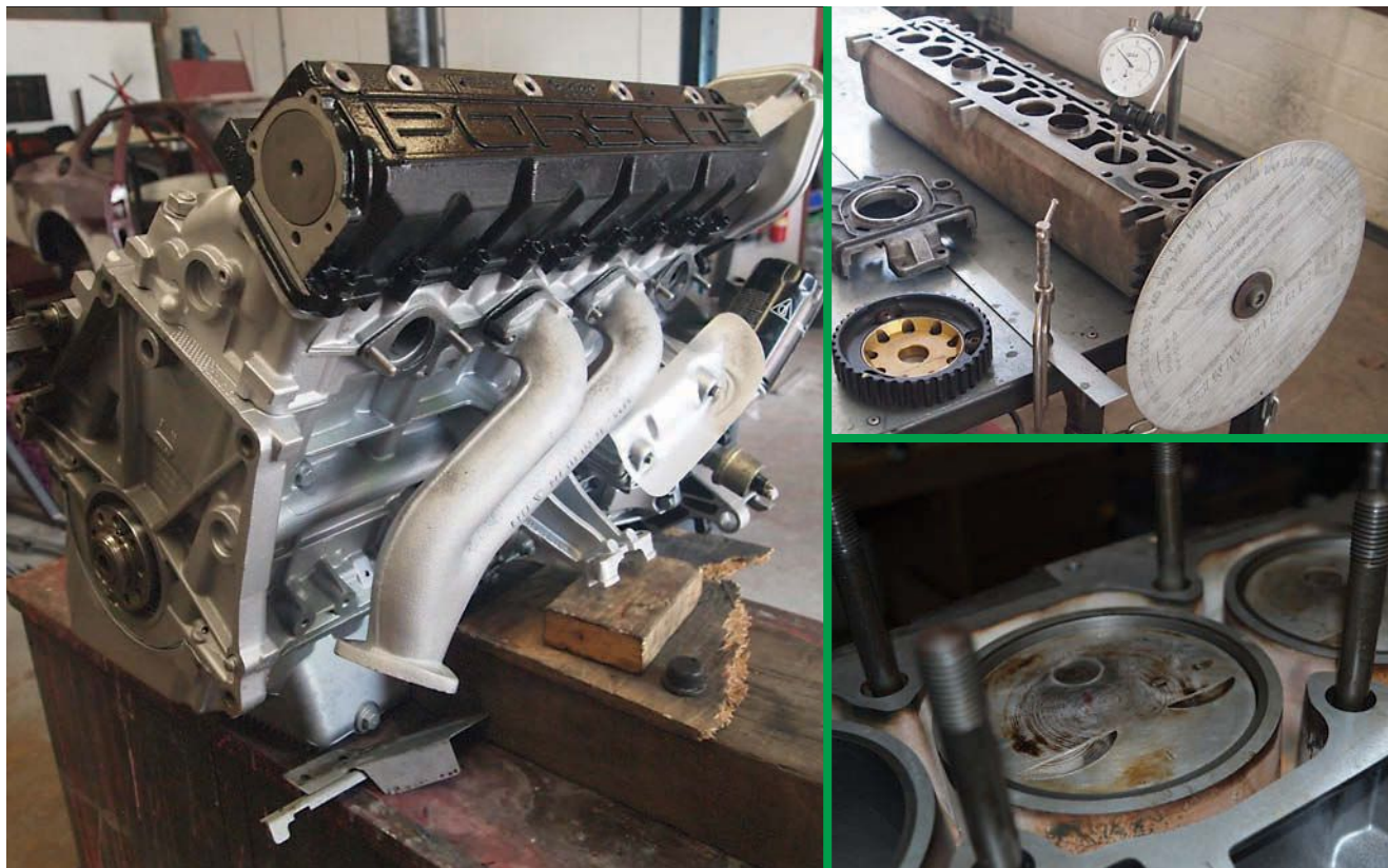
Far left: Check that out! Built-up engine on the bench painted and looking rather splendid with its black cam cover. Left: Cylinder head and cam being 'dialed in'. Below: Pistons sitting snugly in new steel-liner block
