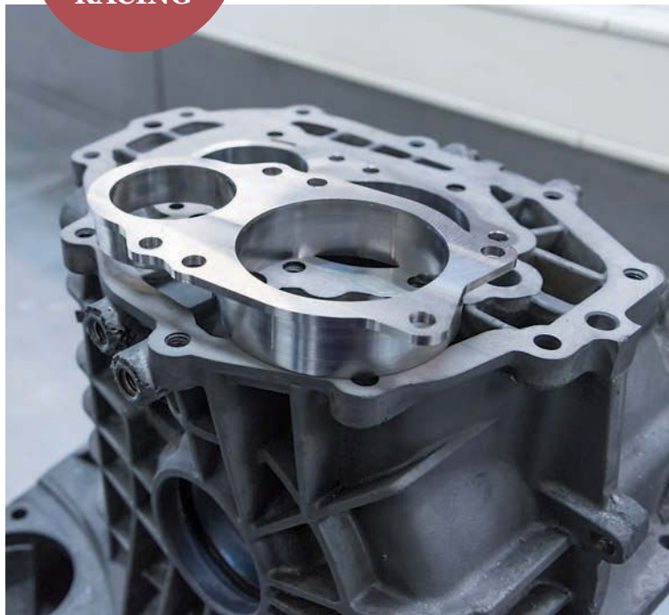
TwinSpark Racing specialise in the 901 and 915 gearboxes, with their own strengthening mods and inserts
