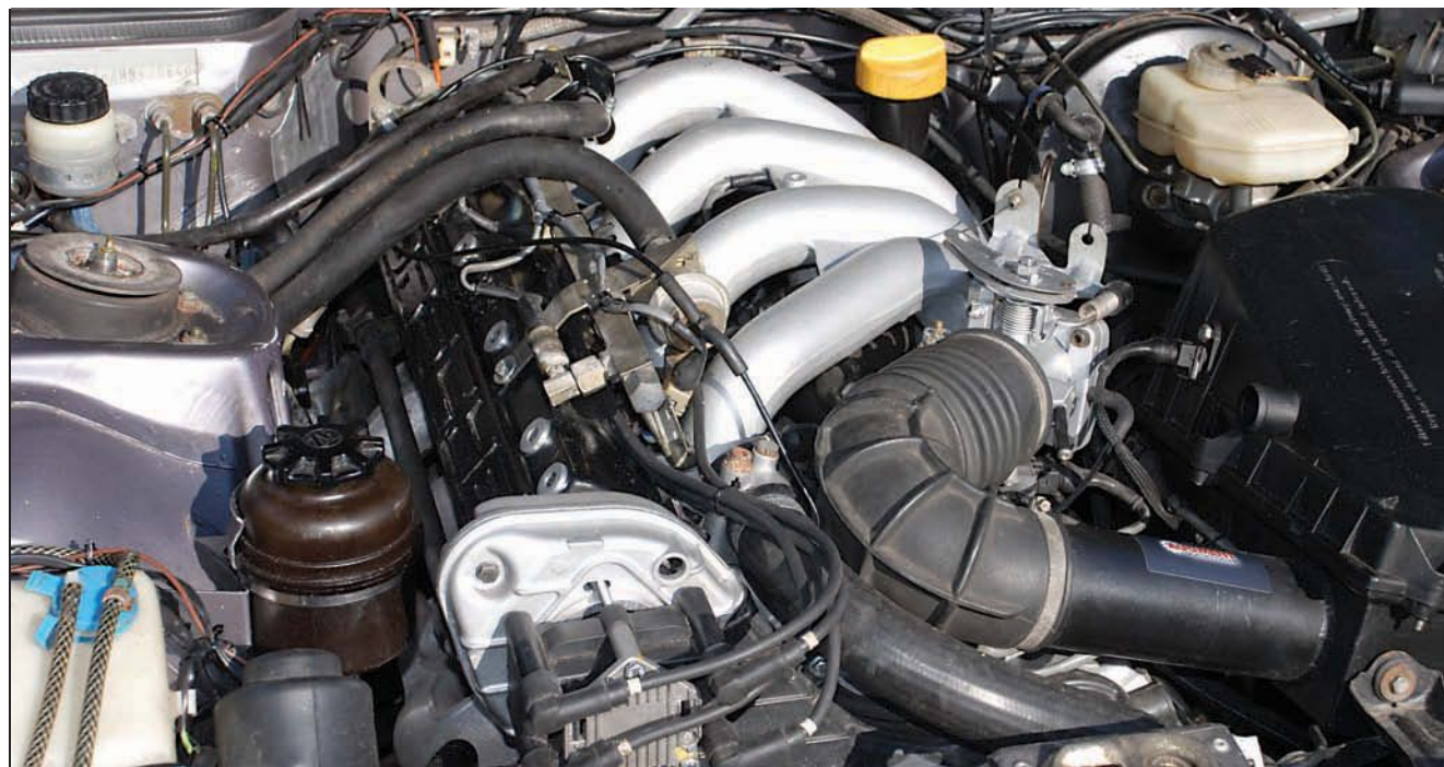
Bay looks rather smart now, with detailed engine. Note the distributorless ignition set up on front of engine and the straight through pipe running from the air box to the throttle body in place of the standard air-flow meter
