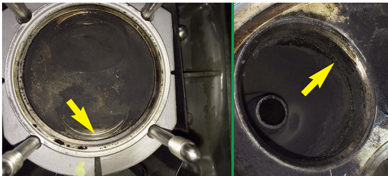
Far left: Arrow points to witness mark on crown of #6 piston, showing where the exhaust valve had made contact
