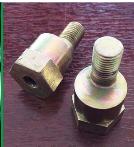
Far left: Front anti-roll bar drop link had play, despite being replaced with one using new Rose-joints. An incorrectly sized mounting bolt was the cause... Middle left: Rear anti-roll bar eccentric mounting bolt (arrowed) was worn, the result of seized Rose-joints Left: The originals were repaired for the MOT but we have now sourced two new ones from Jon Miller of Classic Carreras in Ireland. Thanks, Jon!
