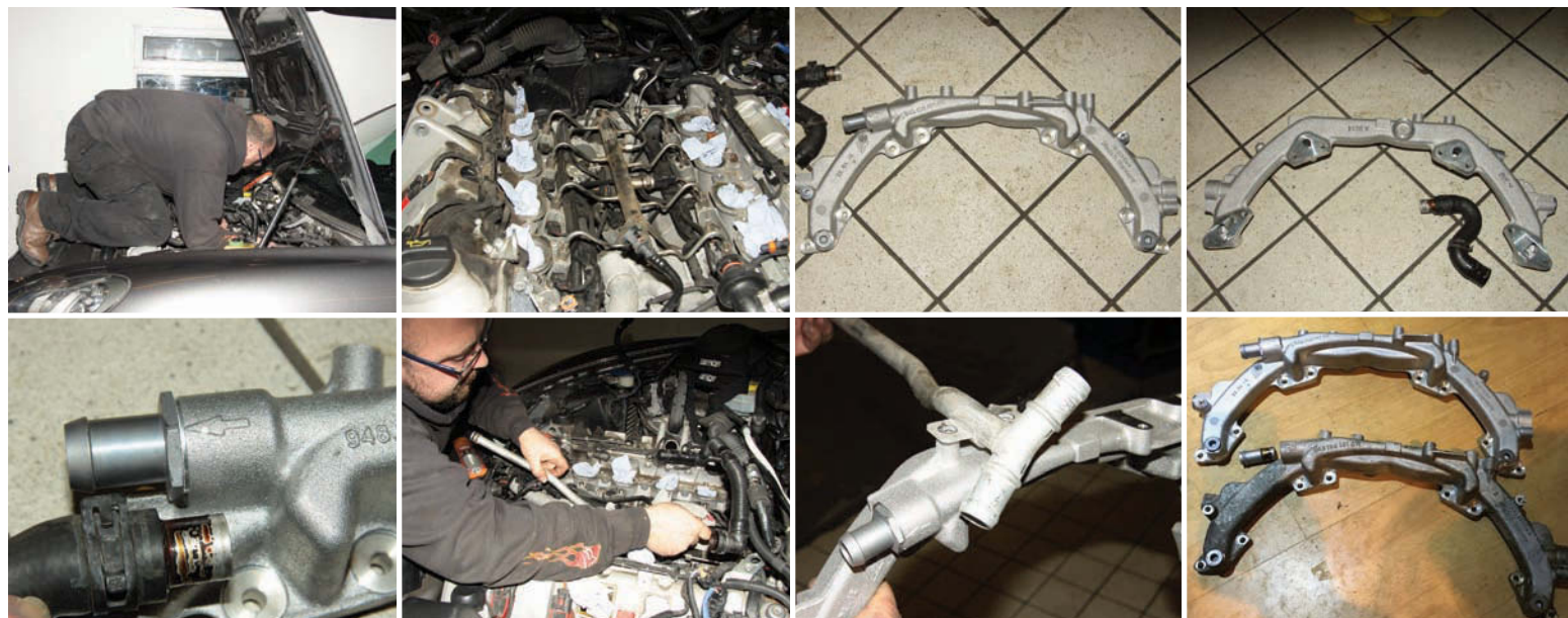
Top row: Kneepads essential. Removing manifold improves access to bridge pipe only slightly. Back and front views of new casting show mounting holes and mating faces with heads, plus hose and failed pipe stub. Above: close-up of new bridge shows how glued-in stub has been replaced with a proper threaded job. Longitudinal pipe prevents bridge being raised, but in the end that had to come off from below, in any case. New and old castings compared: has your car (or the one you are buying) been upgraded?
