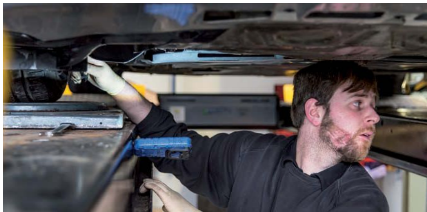
Setting up the geometry. That's the screen that Dan is working from on the right. The trick is to make everything go green!
