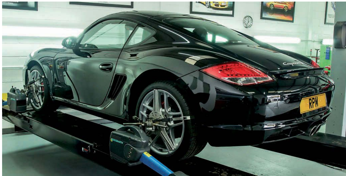
Getting all four wheels pointing in the right direction is essential on a Porsche. RPM use the very latest Beissbarth suspension diagnostic/alignment rig for set-up work
