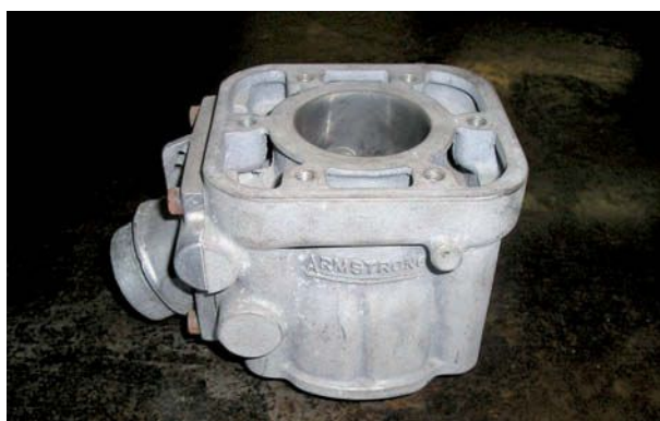
Reduced piston-to-bore clearances extend arc of likely damage. Barry Hart designed this clever closed-deck bike barrel in the 1970s
