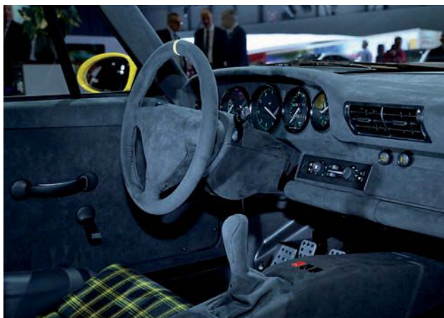
Left: Wow, someone's been busy with the Alcantara! Below: RUF Yellowbird 2017 style. What appears as if it may be a 911 of the 964 variety is actually a carbon-fibre tub and body, with aluminium front and rear subframes. The engine is 3.6-litre Mezger twin-turbo derived and produces 700hp
