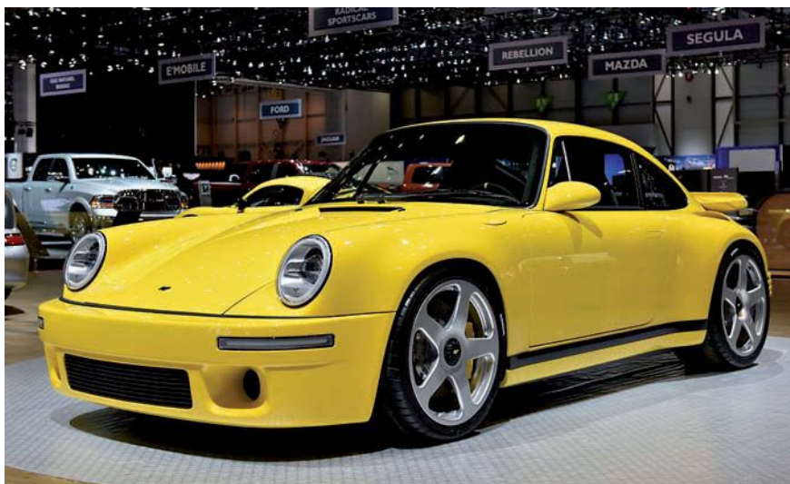
Left: Wow, someone's been busy with the Alcantara! Below: RUF Yellowbird 2017 style. What appears as if it may be a 911 of the 964 variety is actually a carbon-fibre tub and body, with aluminium front and rear subframes. The engine is 3.6-litre Mezger twin-turbo derived and produces 700hp
