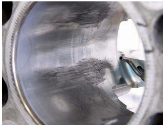
The damage so clearly visible in Horton's own photographs from last year (left and middle) bears a remarkable similarity to that inside the MA1 engines so far examined – in as forensic a manner as possible – by Barry Hart and his team of engineers (this row, right, and top of opposite page). And this is a lot more than mere scoring
