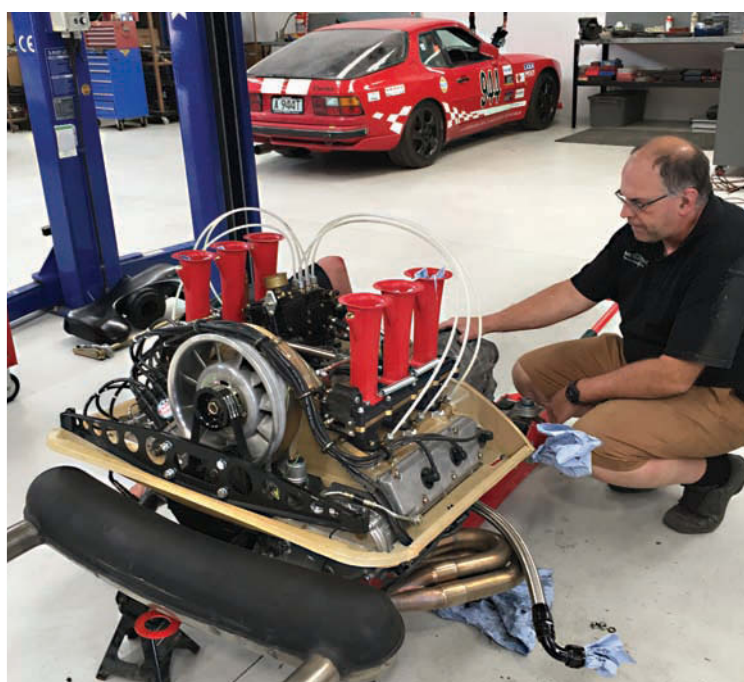
Workshop manager, Iain Langham, with potent 2.8 engine featuring all the right bits including mechanical injection and slide throttle bodies
