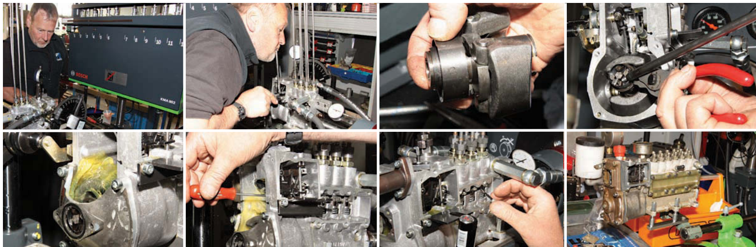
Bosch test-rig at BS Motorsport is capable of setting up six- or 12-plunger pumps – so this 917 unit (bottom row, far right) will be no trouble at all, especially for an engineer as talented and as meticulous as Neil Bainbridge. He has only one arm, but still manages the most taxing of assembly and adjustment jobs – often with the pump running
