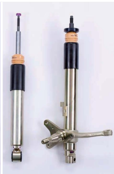
ability to independently adjust the rebound and compression damping settings while on the car will likely be one of its biggest selling points, and it's something that's been achieved through the manufacturer's patented valve technology.
