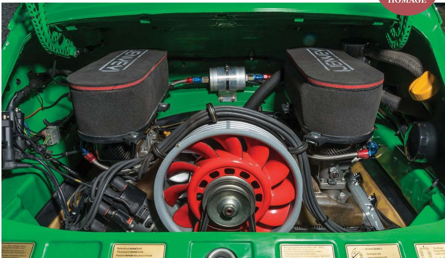
Above: 3.6-litre 964 engine produces 340bhp and 260lb ft of torque. Jenvey throttle bodies and Motec ECU smooth out the wild nature of the RSR 'Sprint' cams
