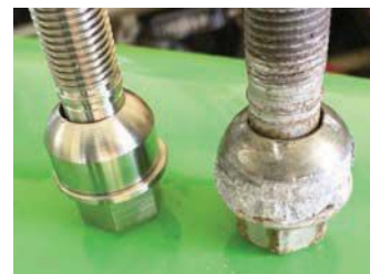
Check your wheel studs. Corrosion can set in and render them a bit useless
