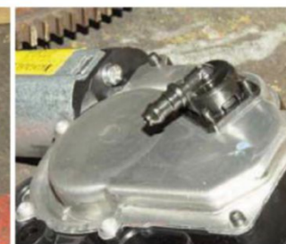
Second-generation Cayenne's rear wiper motor has washer fluid piped through central spindle. Neat packaging, and resulting geometry allows the liquid to be aimed directly ahead of the rubber blade, but blockages in jets can cause it to push past seals, and fill the entire body of the unit. Game over...
