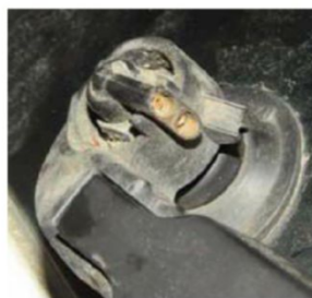
Second-generation Cayenne's rear wiper motor has washer fluid piped through central spindle. Neat packaging, and resulting geometry allows the liquid to be aimed directly ahead of the rubber blade, but blockages in jets can cause it to push past seals, and fill the entire body of the unit. Game over...
