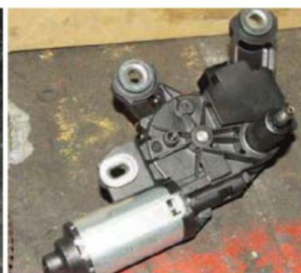
Second-generation Cayenne's rear wiper motor has washer fluid piped through central spindle. Neat packaging, and resulting geometry allows the liquid to be aimed directly ahead of the rubber blade, but blockages in jets can cause it to push past seals, and fill the entire body of the unit. Game over...
