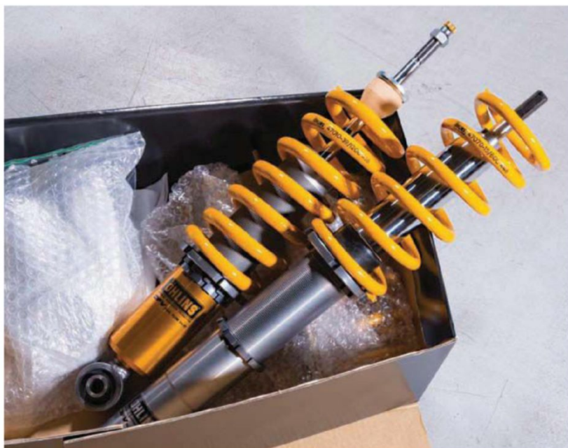
Above: Ohlins coilover kit has prompted this chassis overhaul. Setup and ride height options are numerous. Right: On the road. Ride height is that of Porsche's own X74 sports suspension option
