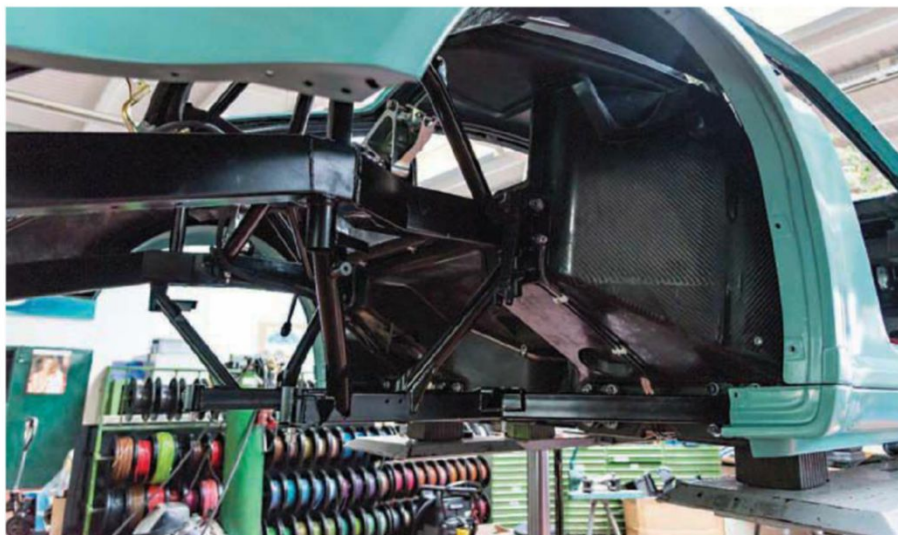
CTR No2 in construction. Note central carbon-fibre tub with front and rear spaceframes attached
