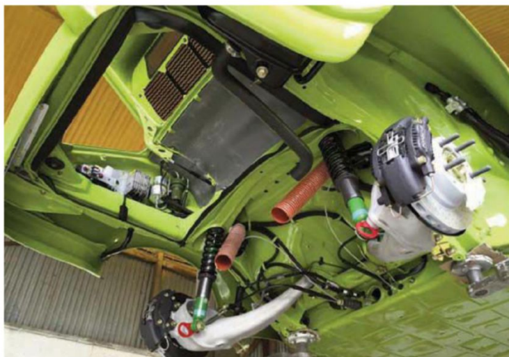
Below, left and right: Level of detailing is impressive, with no component left untouched by Jon's skilled hands. Rebel Racing coil-over suspension conversion is state of the art
