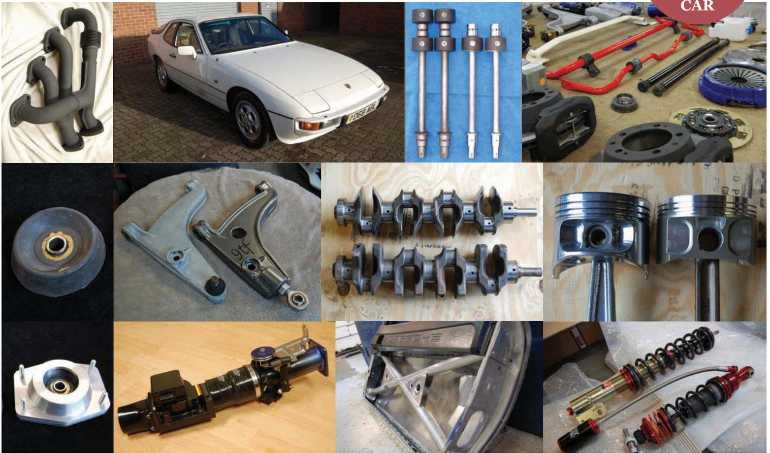
Just some of the parts from this epic build. Starting point was a nice, clean 924S. Lightweight balance shafts make for an eager engine as does lightened, knife-edged crank and lightweight pistons and rods. Note clever, adjustable suspension arms, plus lightweight doors and fabulous Intrax suspension
