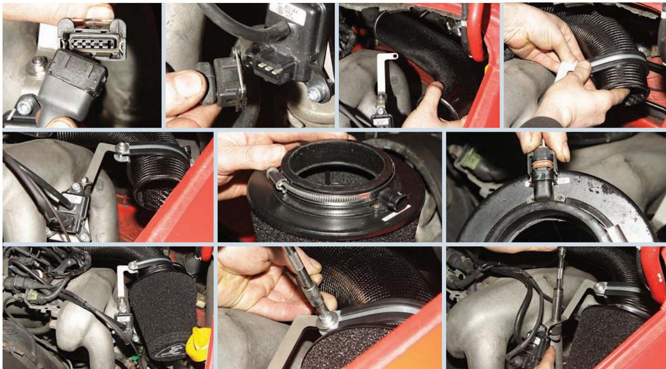
There is a new moulded intake pipe that sits between the air filter and the throttle body, fixed to the MAP sensor's bracket with a large rubber-lined 'P'-clip; as ever in such circumstances, leave all fixings just a little loose until everything is in position and correctly aligned. Don't forget simple plug-in wiring connection to the temperature sensor; it's hard to get at when filter is located on the new pipe. All wiring is supplied, and ready – almost literally – to plug and play
