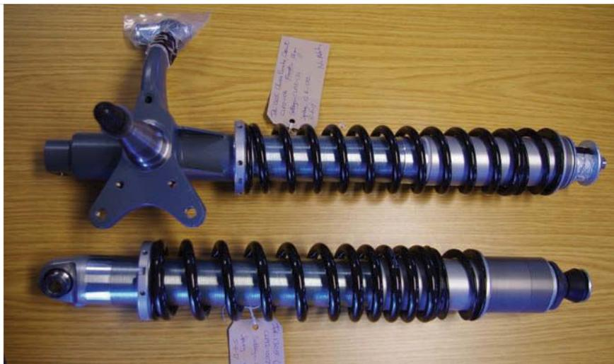
stiffen up before the damper closes completely; because, if you start to run springs which are too soft, obviously there's nothing to stop the wheel going up and you can start to bottom out; if they're nice and soft and you're going over speed bumps, let's say, the wheel will just come straight up, and then anything can happen.
