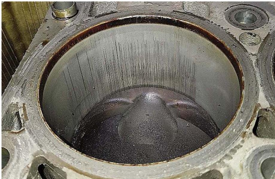
The precise cause of this Gen II 997 failure is – inevitably – debatable, but ASNU's Phil Ellisdon is convinced it's down to something as small and seemingly insignificant as a fuel-injector stem seal
