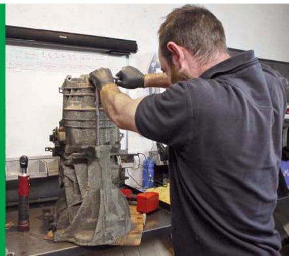
Above: Not only was the clutch done for after 100,000 miles, but the dual mass flywheel was shot, too, so a new one was installed. Right: Commencing the gearbox inspection
