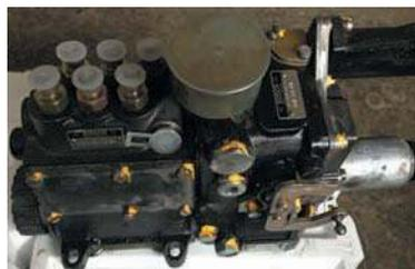
**MFI Bosch fuel injection 010 rebuilt**
