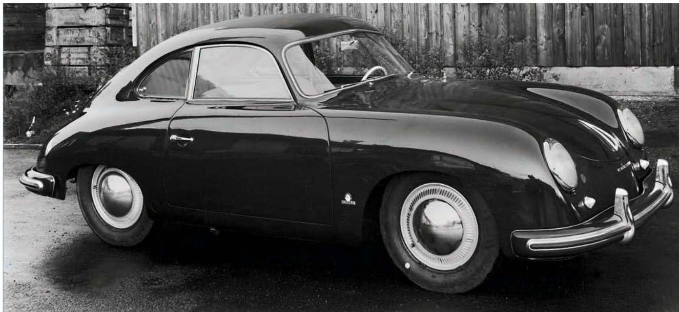
A styling tidy up in 1952 saw the two-piece bent windscreen replaced with a single curved screen. The rear cabin also gained a folding seat
