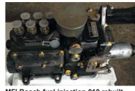
MFI Bosch fuel injection 010 rebuilt Original Bosch MFI mechanical fuel pump for Porsche 911, not used for >30 years, freshly checked and adjusted to actual fuel, deviation <1cm3 for each cylinder. You receive with the pump also full set of documents: test report, copy of owner's manual with description etc, worldwide shipping possible, other parts of private collection clearance available 911-forsale.de. Tel: 0049 15151 829774. Email: cmr2000@web.de (Germany). P0818/050 £3600
