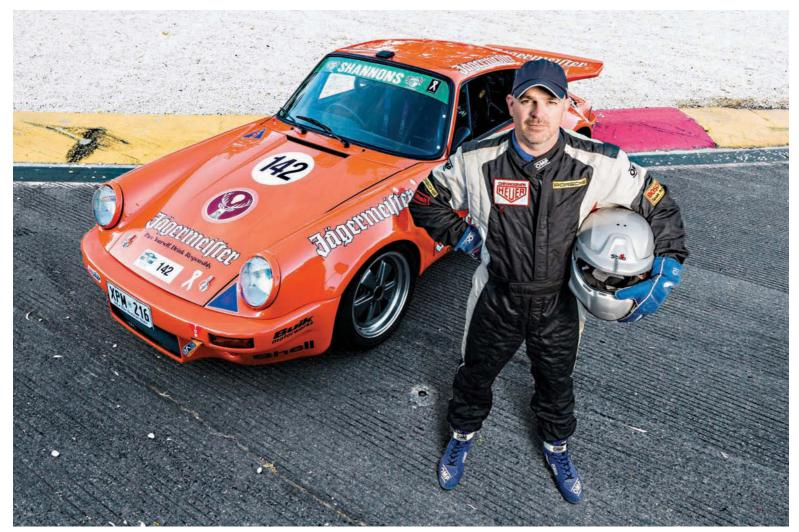
But Tim had what he wanted; front and rear guards, bonnet, rear tail/deck lid and an insert to replace the sun roof, the sun roof having to be removed to allow the fitting – at later date – of the fully integrated welded roll cage from Walker Chassis of Houghton in the Adelaide Hills. And the package had an added bonus. Once fitted, there was a saving of some 125kg. Now the 911 clocked the scales at just 1000kg.
