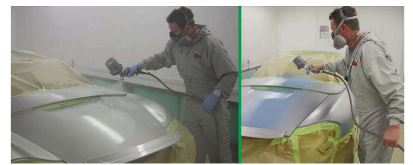
Application is essentially no different to a normal painted respray, with a primer going on first. The difference is, this can be removed entirely to reveal the original paint in perfect condition
