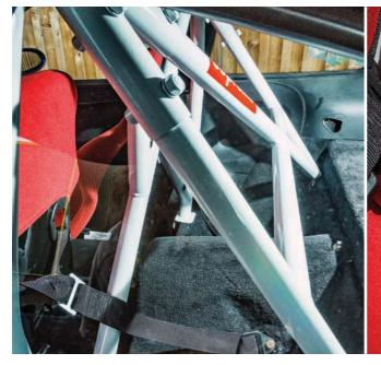
Bolt-in rear cage has been refinished in white, while Recaro Pole Position seats are trimmed in red, the work of Capital Seating in Leicester
