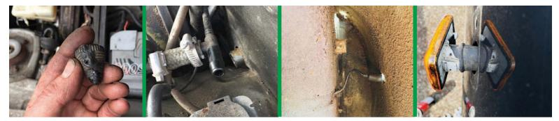
Aerial lead passed through bulkhead via this stepped grommet (above), now filled with mastic sealant and pushed back into hole. Second photo shows where hose to charcoal canister used to connect, in left-hand rear corner of engine bay. View up inside the front wing shows layout of the various components. One annoyance was this broken tab on the indicator repeater lens - these are all rather fragile now
