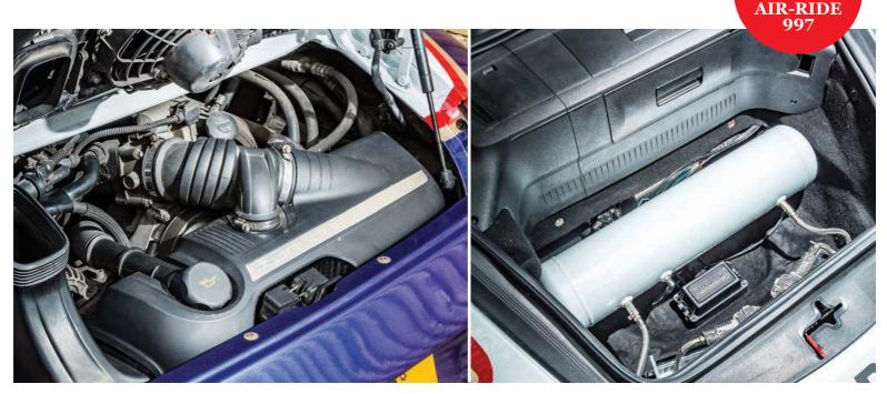
Engine is largely stock, aside from the exhaust system. Front luggage bay is now dominated by the reservoir required by the Air Lift suspension system
