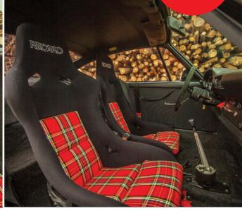
Tartan trim lifts the stripped out interior, while WEVO gateshift lever takes some of the guess work out of the often vague 915 gearshift point harnesses truss driver and co-pilot into the Sparco bucket seats; the driver's seat has fore and aft adjustment but the passenger's is static. A plumbed-in fire extinguisher lives in the passenger footwell, and apart from the Alcantara door liners it's a pukka racing environment.
