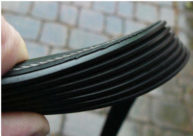
Above: That's some drive belt! Old and brittle, it seemed prudent to change it
