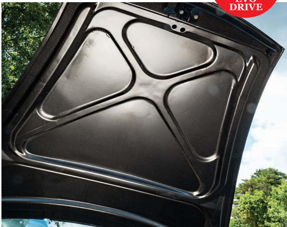
Carbon rear lid with CRS ducktail wing plus carbon bonnet contribute to 45kg weight loss
