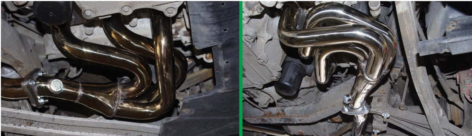
A pipe bending work of art. Shame the new manifolds are hidden under the car
