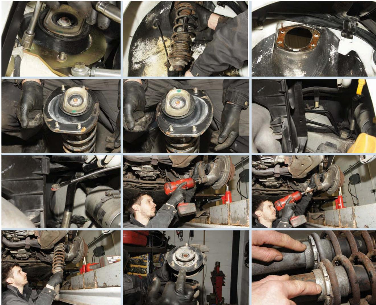
Up top, as it were, the strut is attached to a special mounting plate, itself secured to the body by four M8 nuts (and here with the slight added complication of a transverse brace). Undo them, ideally with an assistant taking the weight of the strut from beneath, and this (near left, top row) is what you will be left with. Brown gasket will need to be replaced, so buy some before you start.
