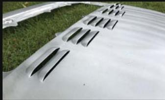
**911 Engine Lids** - These are reproduction brand new aluminium or steel boot / engine lids.
