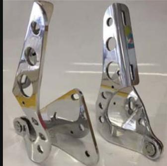
**911 Lightweight Aluminium Bonnet / Engine Lid Hinges** - These hinges weigh in at only 0.7 KG!
