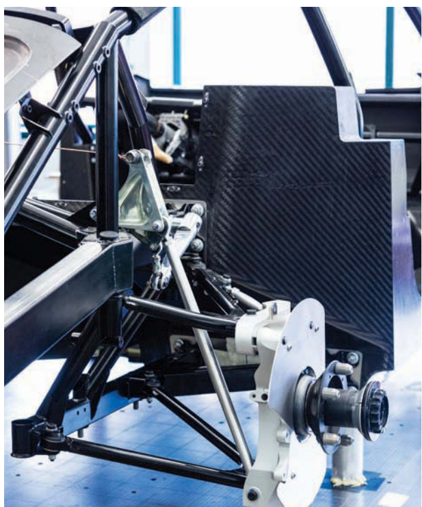
Above: Rear suspension subframe. Right: Yes, it's that light! Alois Ruf happily holds aloft the entire roof section
