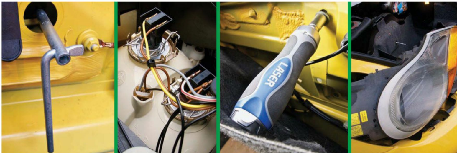
Above: Porsche supply special tool to remove entire headlight unit. Handy. Wiring received a clean up. Best read the story for the full admission of bulb changing muppetry
