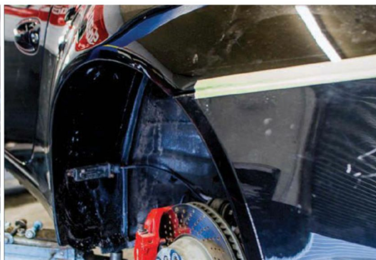
Below: Olly's 997 is part way through a wide-body overhaul – the wheelarches being sliced and sectioned in steel to provide a subtle, yet moody appearance
