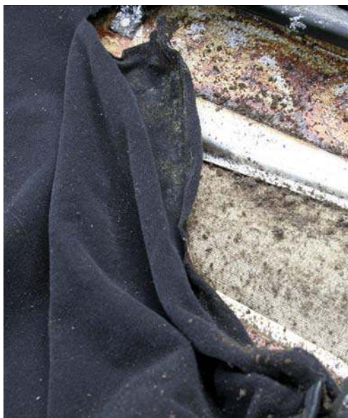
Pulling away the old headline reveals its poor state, and also the accumulation of dirt and old glue. Note also the poor condition of the roof perimeter frame
