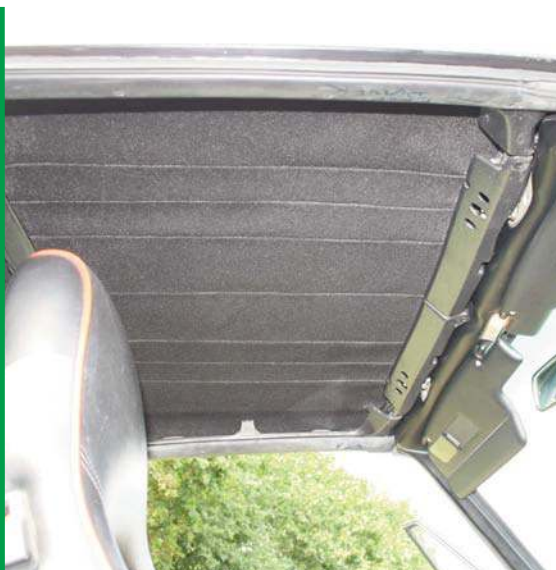
Targa top back where it should be! Note neat fitting headlining and the Hammerite re-painted perimeter frame. Now I'm waiting for rain and a good run to see if it leaks
