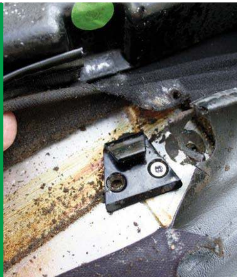
The clip bolts on the front edge of the frame were rusted to their screw plates and had to be drilled out. Rears were not rusted and came off easily
