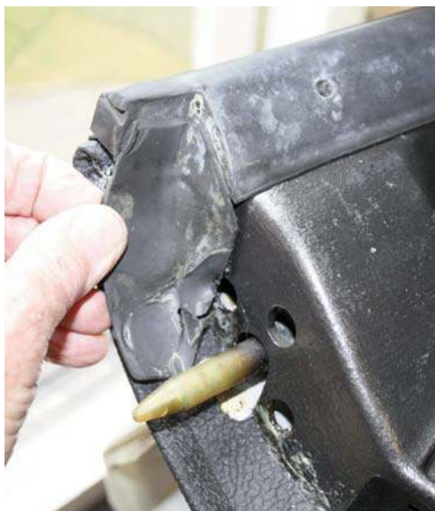
The window seals and gutters are fixed to the frame and the seal ends (tatty, new ones unobtainable) are glued in place and the end plates fitted
