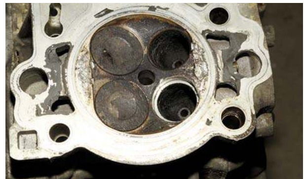
It's the classic Catch-22: M96 valve seats could drop out at any time, but there's no way of telling until they do. Either way, any cylinder-head work should now include their replacement
