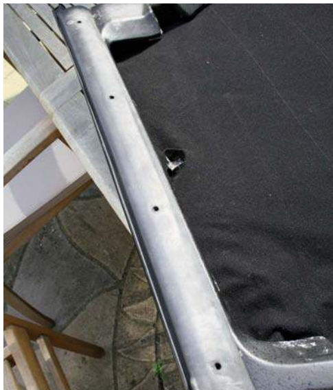
The lateral window seals are fixed to the frame sides and held in place by self-tapping screws accessed through the holes. The steel 'gutter' is still in place
