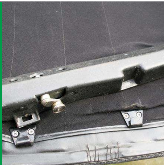
Front and rear hinged frame parts locate in clips which are bolted to the roof plates and also help keep the leathercloth and headlining in place. This is the front
