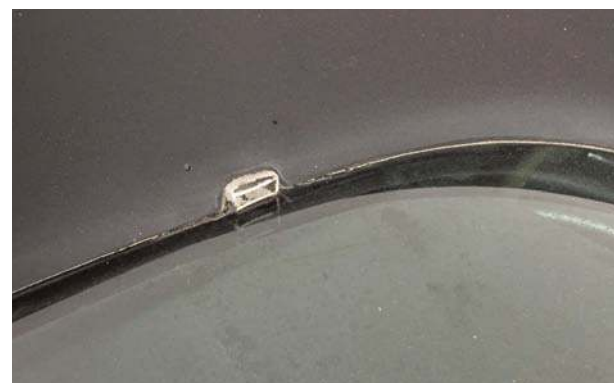
Whether this tube – and the one on the other side – keep 924's rear-spoiler drain holes clear is hard to say, but they must help
