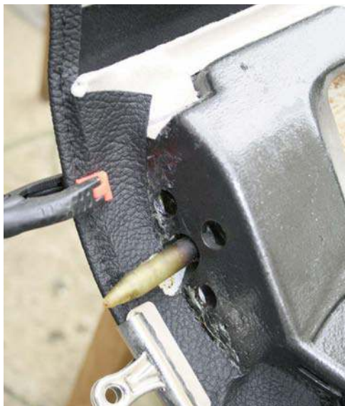
Once the leathercloth has been stretched over the top it is glued to the underside of the frame. Corner pieces need clamps to keep them in place
