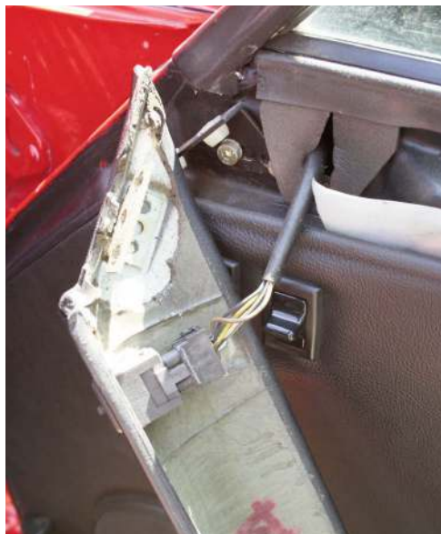
To get at the window mechanism the door trim has to come off. The capping strip is secured by screws at both ends and contains the joy-stick for door mirror adjustment. Note the top bolts for the door pull on the right
