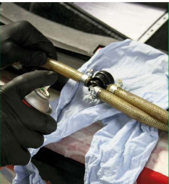
Hose tidied up (ie: split bit cut off), new valve and clamps fitted before giving a quick squirt of underseal protection
