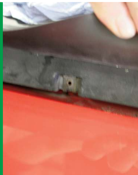
Rubber 'smile' between body and front bumper can be partly released by bending up and releasing a couple of screws...
