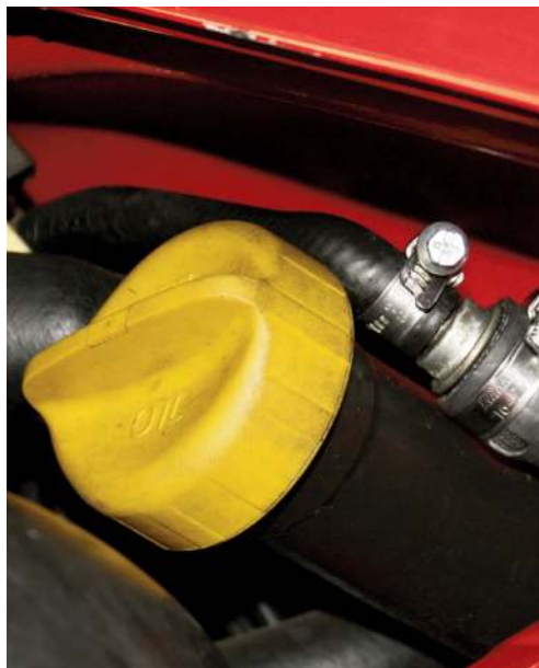
Short breather hose to top of oil filler within the engine compartment was replaced
