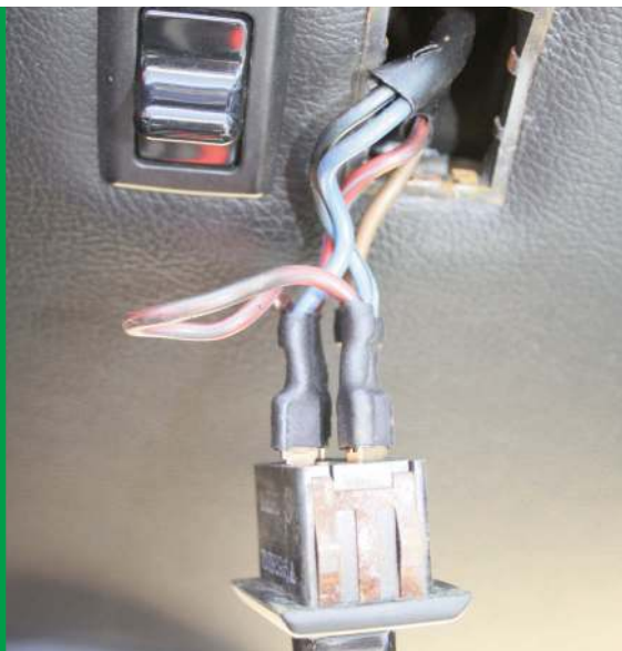
The window lift switches have to be prised out from the main door trim
