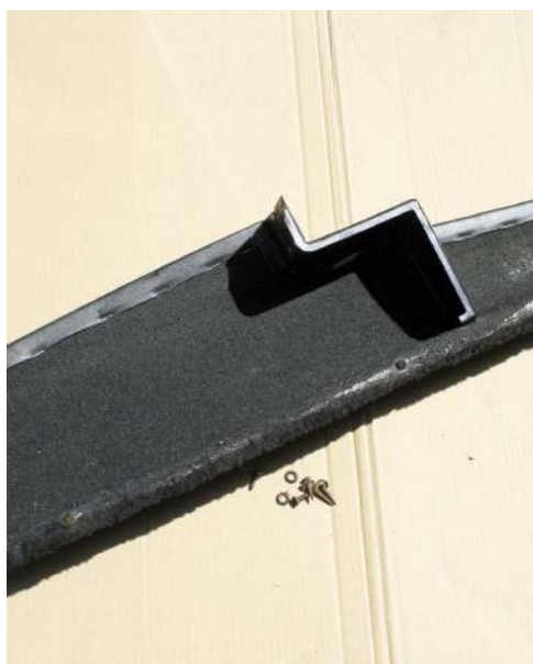
The door pocket is held by self-tapping screws through the door trim and also to the door pull
