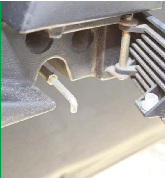
The door opening catch has the operating rod located in a nylon bush on the pull handle. Prise out carefully to avoid damage
