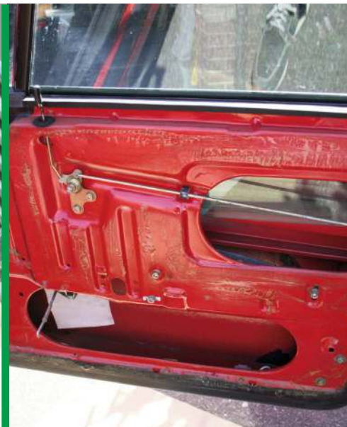
Once the central locking knob has been removed (one bolt under the knob trim) the door card, held firm by self-tapping screws, can be removed. At this stage the speaker wires will have to be disconnected
