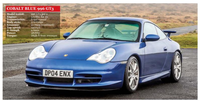
rest of the 996 range, Porsche released the second generation GT3, which became widely referred to as the 996.2 GT3. To the casual observer, there were few differences, the most noticeable of which were the redesigned headlights (no more fried eggs...) and a switch to using the bodyshell of the Carrera 4. Under the skin, though, there were six-pot brake calipers used at the front (with
