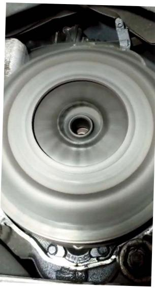
There is a not inconsiderable amount of work involved in removing a 996 gearbox (see last month's how-to story) and then enabling the engine to be run such that one can (hopefully!) track down a mysterious noise, but desperate times call for desperate measures. Here, with the clutch still in place, the light tinkling noise sounded to us very much like a timing-chain problem
