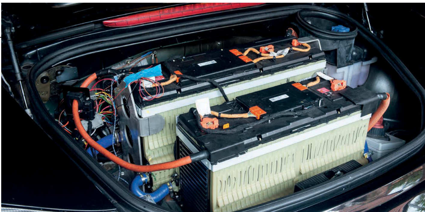
Bulk of the batteries are in the boot. They're from a Vauxhall/Opel Volt. As battery tech improves, then they can easily be replaced
