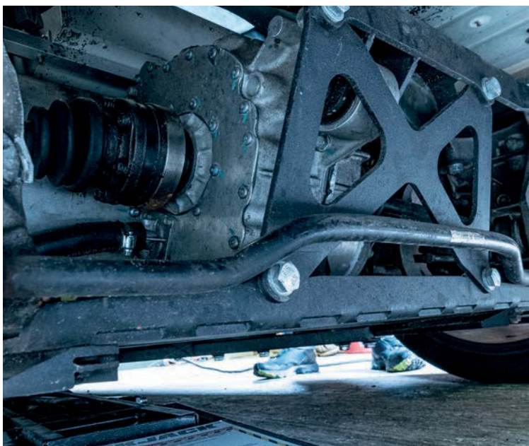
Paul built a subframe to carry the compact Tesla motor. Handily, the motor and differential is all one unit. Right: High-voltage junction box and further batteries live under the engine cover
