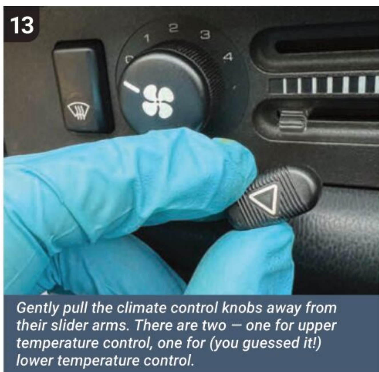
You can now pull the climate control fascia panel free. It's a thin piece of plastic and quite fragile, so exercise restraint. You might find the panel sticks at one end. Go grab your trim removal tools.
