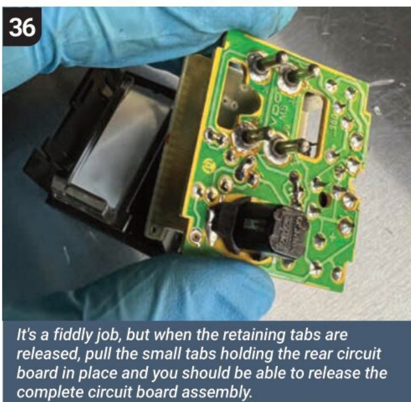
The remaining clock components might break free when you remove the circuit boards. Other than the knackered screen, we need to reuse all of these parts, so keep them safe.
