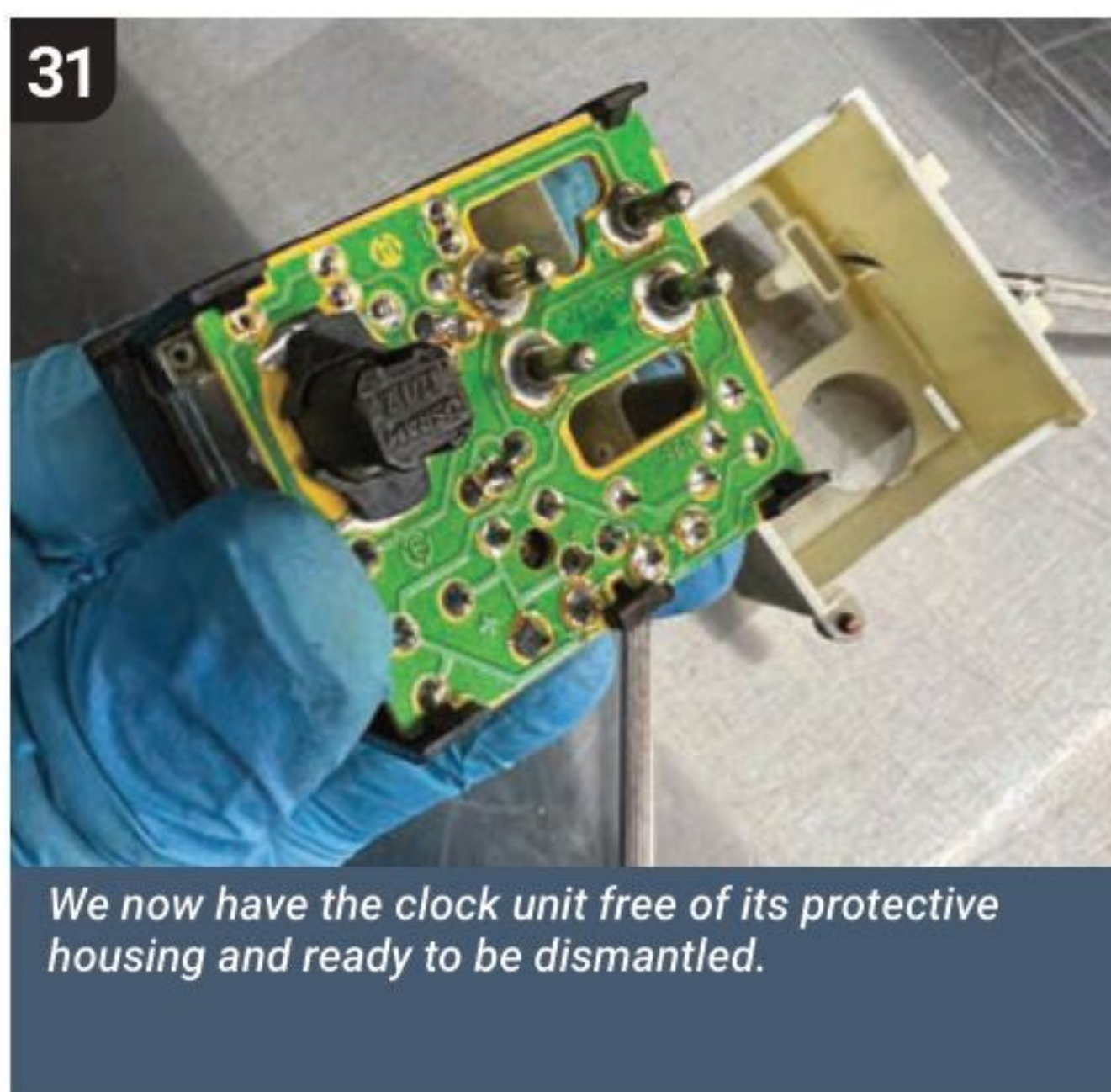
Here we see the overall structure of the clock. There are two circuit boards (one top, one bottom) soldered together. The clear plastic lens reflects light from the bulb, illuminating the clock.
