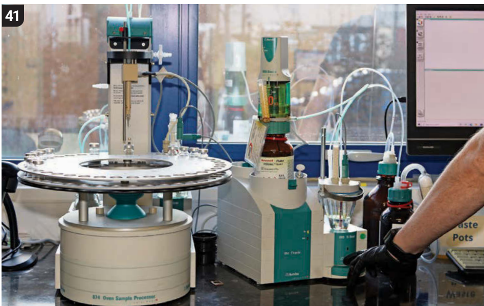
41 While the crackle test (steps 10 and 11) checks for excess water, The Karl Fisher Test machine establishes the quantity of dissolved moisture present. Engine oil is designed to keep a degree of engine water in suspension, largely to reduce the chance of it separating and being sucked up by the oil pump (instead of lubricant).
