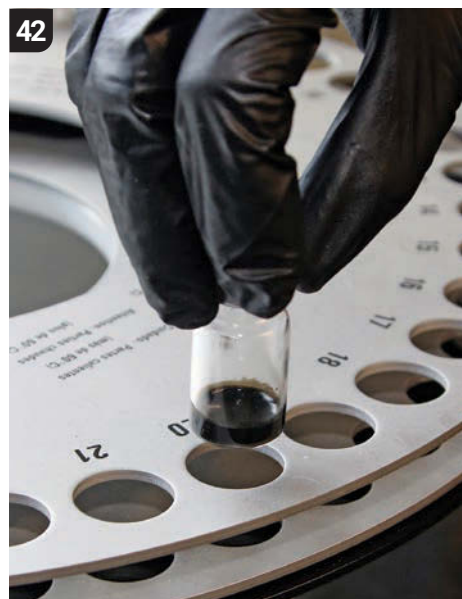
42 A known weight of oil is measured and placed onto the machine. The oil is then heated in order to evaporate the water suspended within it.
