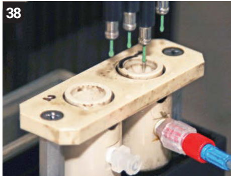
38 Once the process has been completed, the machine engages a strict cleaning process, which flushes all pipework with heptane solvent and discards the tip.
