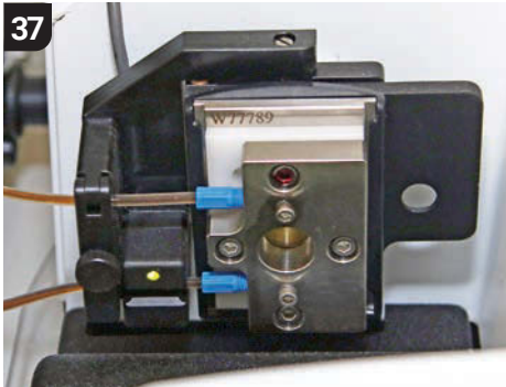
37 A vacuum pump draws the sample into a 0.1mm thick gap between two small plates of transparent glass. Infrared light is then shone through the sample to calculate its structure.
