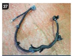
The new wiring harness ready for installation. You may find it useful to have a friend help route the cable around the oil cooler and down the side of the gearbox while you feed it through from above.
