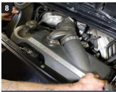
Wiggle while you work and lift the airbox away from its locating pins. Make sure the loose jubilee clip doesn't fall into the engine bay and be careful not to cause damage to the oil filler neck.
