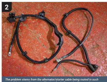
The problem stems from the alternator/starter cable being routed in such a way it is exposed to repeated heat cycles in the engine bay, causing deterioration. A new genuine cable (pictured left) costs £116 from Design 911 (design911.co.uk) and the fix should take no more than a few hours. Look for part number 99760701903 (manual) or 99760701804 (Tiptronic).
