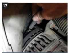
And here is where the connector attaches to the back of the alternator. With the unit pulled forward, access should be easy enough, but you will need to get a ratchet and 13mm socket in there.
