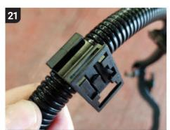
The alternator/starter wiring harness is held firmly in place by a pair of clips attached to engine bay hardware. These are notoriously difficult to see, but need to be unfastened to allow removal of the cable.
