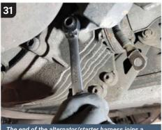
The end of the alternator/starter harness joins a second loom routed all the way along the car to the battery. In some cases, this loom may also need to be replaced, but can be treated as a separate job.
