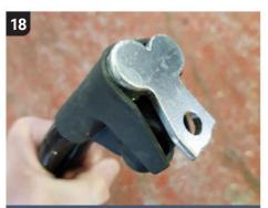
This is the connector linking the wiring harness to the starter (refer to step 2 of this guide for clarification). The heat of the engine bay can cause the rubber boot to melt, leading to problems.
