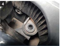
The main body of the airbox is held firm by locating pins. You will require no tools to pull the part free, but exercise care and be sure the following steps are observed beforehand.
