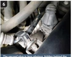
The second plug is less obvious, hidden behind the airbox body, but easily accessible. Pince the locking pin and disconnect the plug. Pull it to one side.
