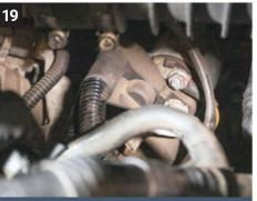
Here is the same connector, as viewed from within the engine bay, and with the harness attached to the starter. Access is limited, so unscrew using a 13mm socket on the end of a universal joint.
