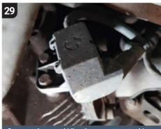
Return to the cover hiding the connector attaching the wiring loom to the side of the gearbox. Undo the two 10mm bolts.
