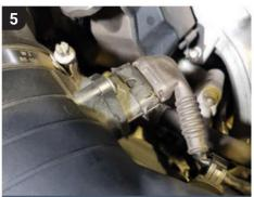
There are two wiring harness plugs attached to the airbox. Both need to be disconnected and pulled to one side. The first is clearly visible on the back of the housing. Carefully pull it free.
