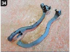
The removed plastic cowling. As noted, the smaller dimensions of the 997's manual transmission allows for easier harness removal and installation, meaning the previous step may not be required.
