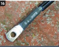
This is the wiring harness connector attached to the rear of the alternator. It can be a pig to get at unless you have sufficient lighting and nimble wrists, even though removal is a case of simply unscrewing a nut.
