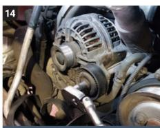
The harness we're replacing is attached to the rear of the alternator. We need to pull the unit forward to get access, which means removing the auxiliary belt. Using a socket, loosen the idler pulley.
