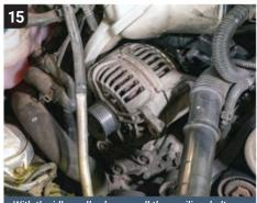
With the idler pulley loose, pull the auxiliary belt free, unscrew the alternator's fastening bolts and pull the unit forward (you may need a pry bar), thereby allowing access to its rear.
