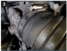
To begin with, raise the car on a ramp or axle stands. Remove the scuttle covers and disconnect the battery. Then, remove the airbox. Begin by loosening the jubilee clip fastened to the throttle body.
