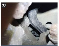
Shine a light where the alternator/starter harness lives and you will see the plastic cowling. Its rigidity can make cable extraction through the engine bay tricky. Separate the cowling from the harness.
