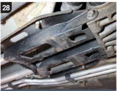
This picture illustrates the mounting bracket attached to our Tiptronic S-equipped 997's gearbox. Undo the six 16mm bolts holding it in place and the transmission will drop a few millimetres.
