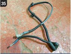
The removed alternator/starter harness. At first glance, there doesn't seem to be much wrong — no sign of cable damage and the rubber boot is in tact — but heat can deteriorate wiring hidden from view.
