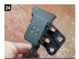
This end of the alternator/starter harness attaches to the gearbox. It is hidden from view, and the plastic cover hides a fastening nut, which must be removed to allow the old loom to be pulled free.
