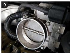
With the airbox dismissed, you can now remove the throttle body. Four bolts hold the part in place. Use a ratchet and socket to unfasten all four.
