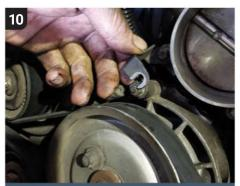
There is a mounting support bracket attached to the throttle body. It needs to be removed, but undo the bottom nut with care — it is paired to a fixed bolt with an integrated rubber collar prone to splitting.
