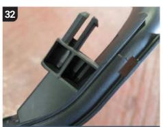
The harness we are removing (and the one were are installing) features a plastic cowling to force routing and to protect the cable from corrosion. This locating lug is pushed into the gearbox housing.
