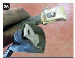
These are the connectors previously attached to the back of the alternator and the starter. Yours may show serious corrosion or melted rubber. Signs of failure, however, aren't always so obvious.
