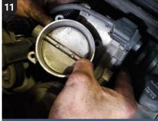
Undo the wiring harness plug attached to the throttle body and pull the part clear. Now is the perfect time to clean it free of any contaminants, such as build-up of sticky oil between the housing and butterfly valve.
