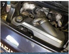
With the two wiring harness plugs disconnected and the jubilee clip fastening the airbox trunking to the throttle body loose, it is now possible to pull the airbox free.
