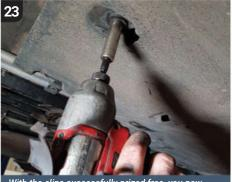
With the clips successfully prized free, you now need to work underneath the car. Using a 10mm socket, undo the plastic nuts holding the protective undertrays in place and pull them free.
