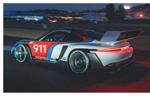
the 24 Hours of Daytona in 1978. The 4.2-litre six-cylinder boxer engine (a power unit revving to 9,400rpm) achieves output of as much as 148bhp per litre of displacement, likely a record for a normally aspirated GT race car, making it significantly more powerful than when fitted to the GT3 R, which develops up to 565bhp (depending on restrictions imposed by an event's Balance of Performance).
