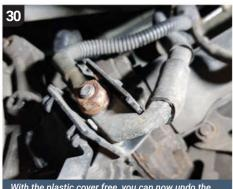
With the plastic cover free, you can now undo the 13mm nut holding the wiring harness in place. The position of this nut makes it susceptible to corrosion. Renew the part, rather than reinstalling.
