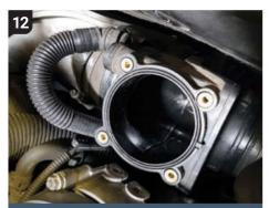
Next up, you need to remove the plenum behind the throttle body. Unclip the breather hose and then loosen the jubilee clips attaching the part to the main intake pipework. When loose, pull free.
