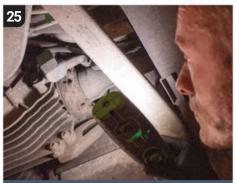
With undertrays removed, this image shows you where the harness attaches to the gearbox. If working with a Tiptronic, the transmission will need to be slightly lowered to allow enough room to work.
