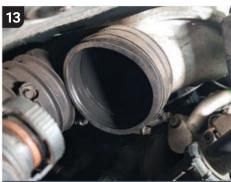
If you've excessively loosened the jubilee clips attaching the plenum to the main inlet pipework, put them to one side or re-tighten them to ensure they don't drop down the back of the engine bay.
