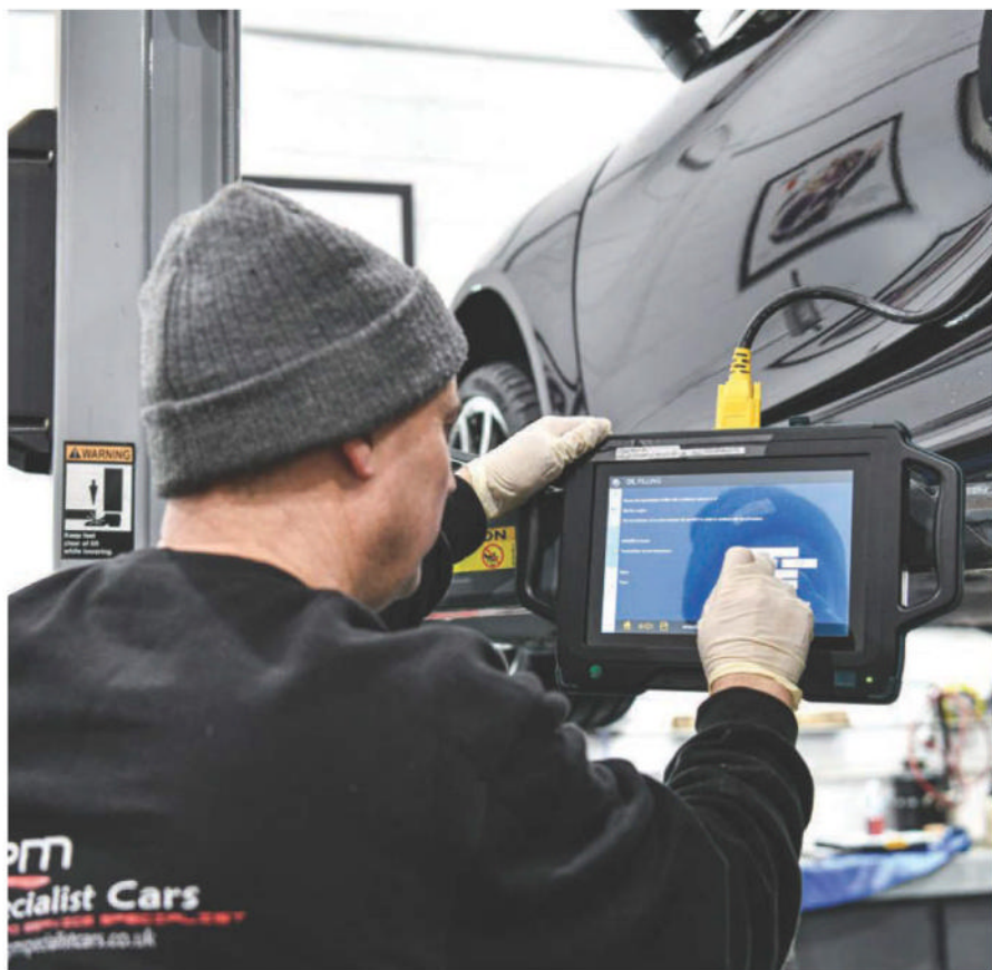
Above Recalibrating PDK's dual clutches
