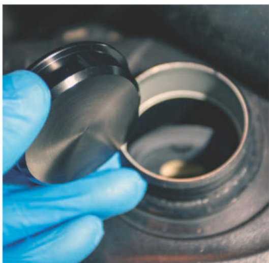
Above Replacing the rubber resonator pipe delete cap with a hard anodised aluminium part
