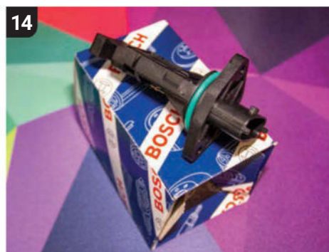
14 We highly recommend fitting a new mass airflow sensor (part no. 98660612502) when installing a Fabspeed intake system. If not, you will need to remove the old sensor from the standard air box.
