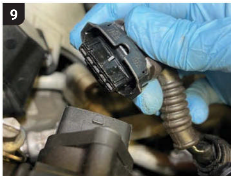
9 The mass airflow sensor plug is easy to see. Carefully unfasten it from the sensor and pull the plug to one side.
