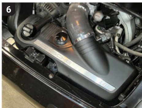
6 Obviously, the first thing we need to do is remove the standard air box.
