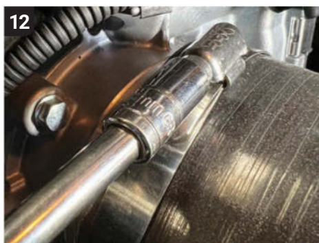
12 Take either a flat-headed screwdriver or the appropriately sized socket and loosen the jubilee clip holding the intake pipe to the throttle body. Then, pull the pipework away from the throttle body.
