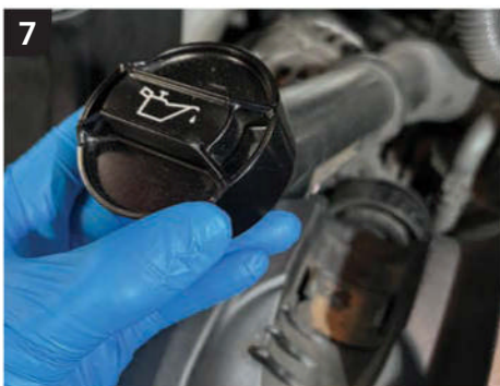
7 Lift the oil filler neck free of the air box and rest it to one side.
