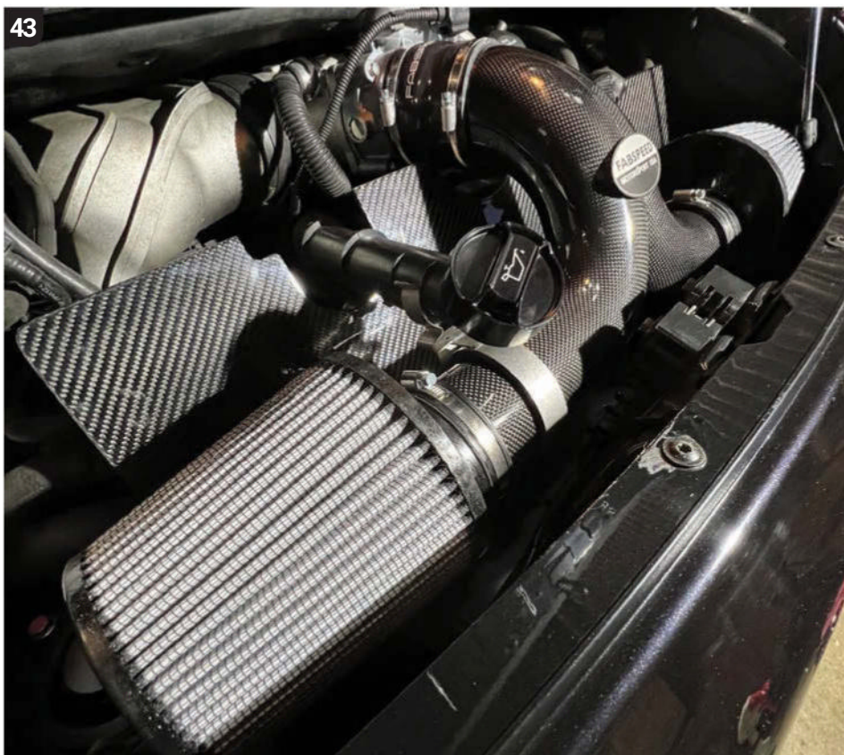
CAD-designed for maximum airflow, Fabspeed's carbon-fibre competition intake for the 997 looks great, sounds great and releases trapped power. Expect to see a road report in a forthcoming issue of 911 & Porsche World.
