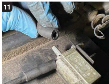
11 You'll note vacuum piping feeding into the solenoid from the engine bay. Carefully pull the pipe away from the solenoid.
