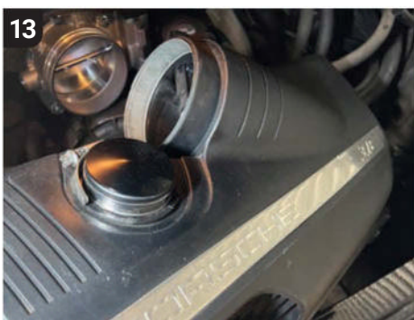
13 If the intake pipe is silicone, you may need to loosen the jubilee clip attaching it to the air box. Pull the air box toward you and lift, but be careful not to scratch it on the engine lid lock latch.
