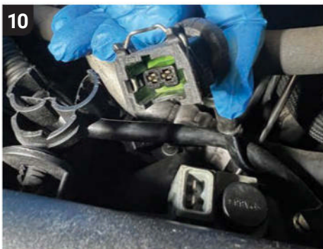
10 The second plug is less obvious, hidden behind the air box body and attached to a vacuum solenoid, but easily accessible. Pince the plug's locking pin and disconnect it from the solenoid.
