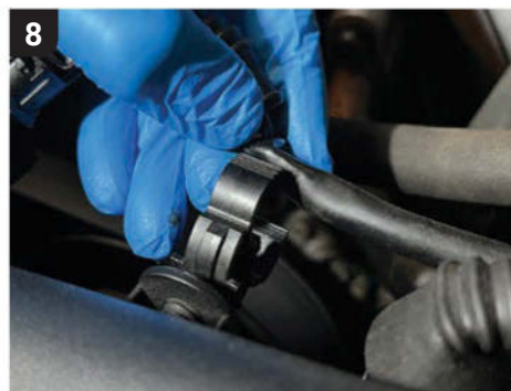
8 There are two wiring harness plugs attached to the rear of the air box. Both need to be disconnected. Open the clips holding each plug's wiring in place.
