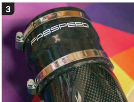
3 Fabspeed offers its carbon-fibre competition intake system with the option of a silicone GT3 throttle body adapter for 997 Carrera engines upgraded with the GT3's 82mm throttle body.
