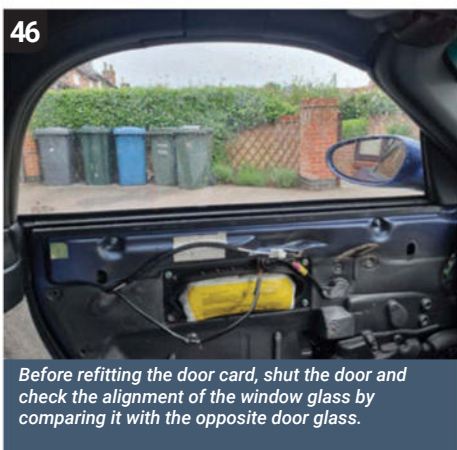
If alignment needs to be altered, use these torx adjusters on the window regulator to raise or lower both the front and rear edge. The adjusters can be accessed via grommets under the edge of the door.
