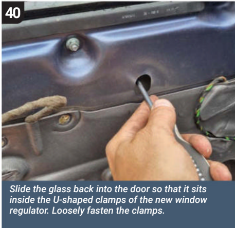
Lower the window into the door frame and check the rubber lining of the clamp sits on both sides of the clamp itself. Loosen the bolts, align the glass on your pen marks and tighten the T30 torx screw.
