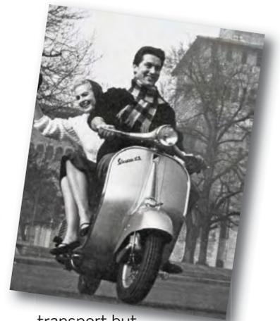
transport but a vehicle meant for leisure. The GS reached 100km/h, it was the first Vespa with a 4-stroke engine, a two-seater saddle and handlebars in die-cast aluminium. At the launch, Piaggio caught its competitor Innocenti completely unprepared.
