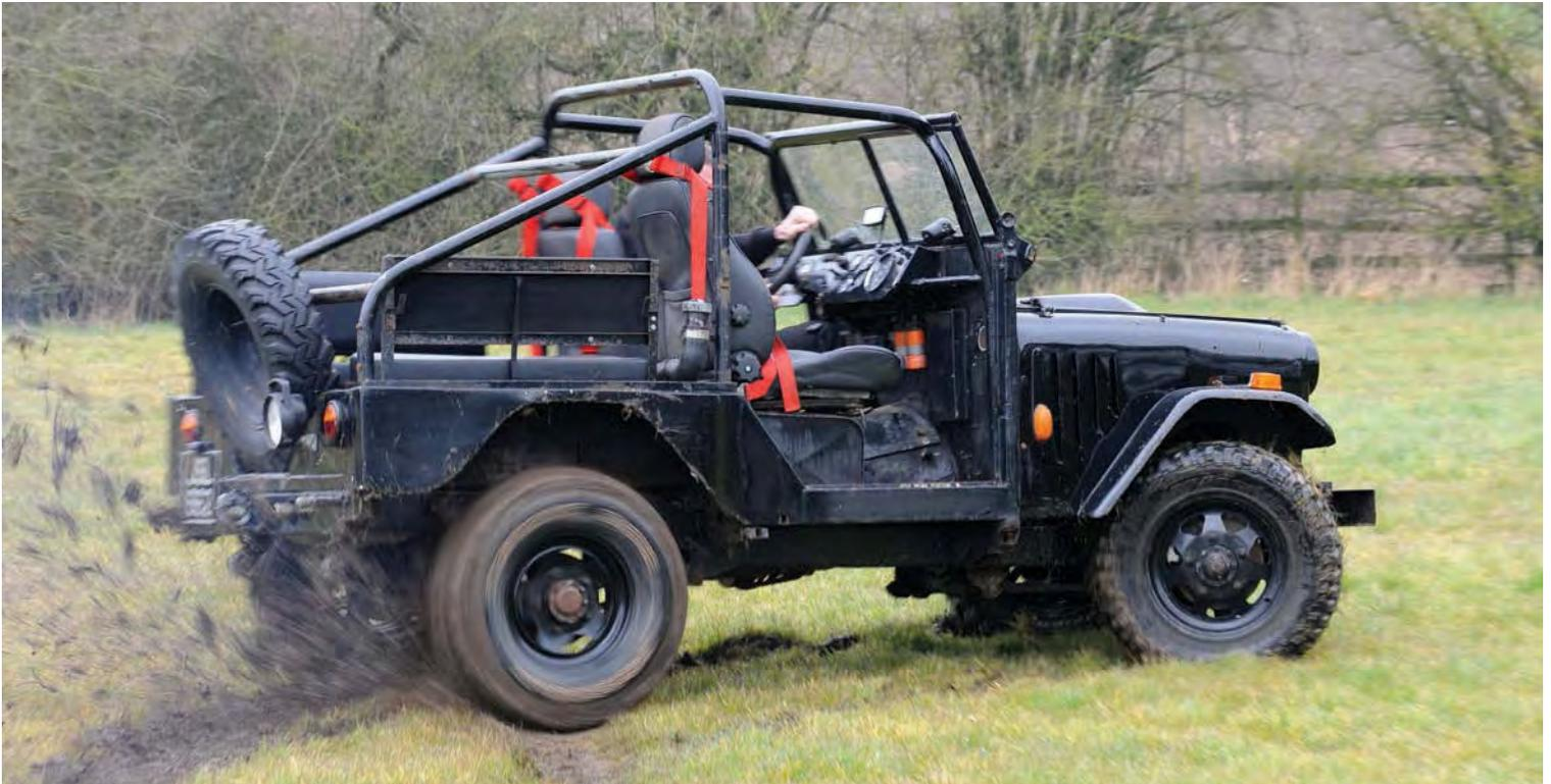
absorbers which significantly improve the ride and off-road ability. A hydraulic diff locks front and rear instead of cable operated ones found on a standard Matta. Alfa 156 leather front seats and a set of rear bench seats from a Land Rover have been fitted for ease of cleaning when it gets really muddy
