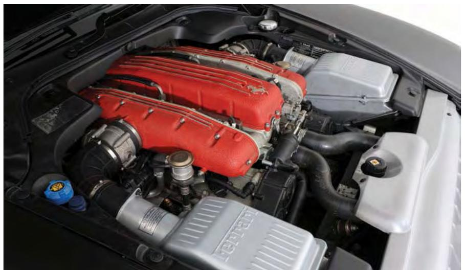
*The 5.7-litre V12 sits well behind the axle line, the front mid-engined layout providing advantageous weight distribution*
